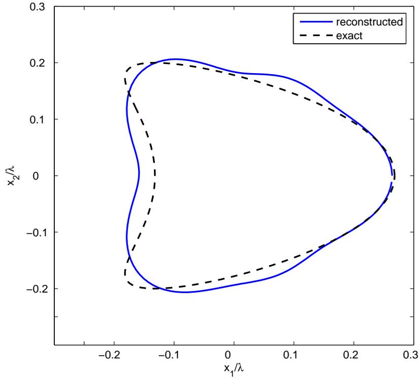
**Figure 5.12:** Exact and reconstructed geometries of a kite-shape object
