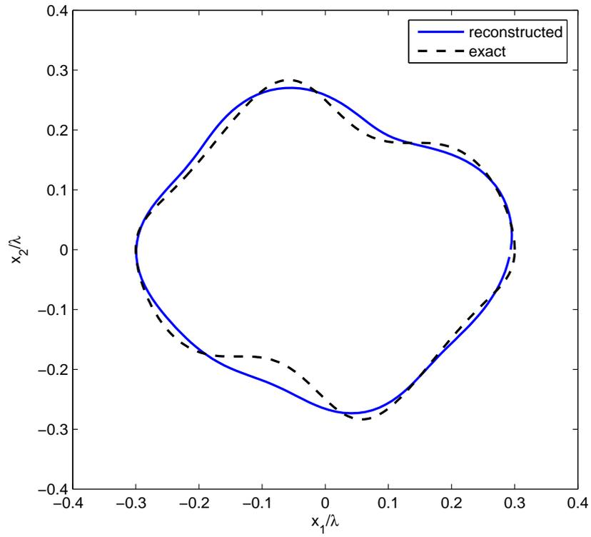
**Figure 5.1:** Exact and reconstructed geometries of a potato-shape object for  $\varepsilon_r = 4$
