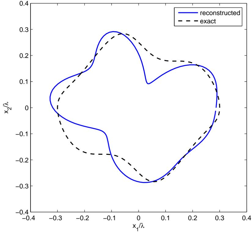
**Figure 5.9:** Exact and reconstructed geometries of a potato-shape object for the radius of the  $\beta$  is 25% greater than  $f_{max}$
