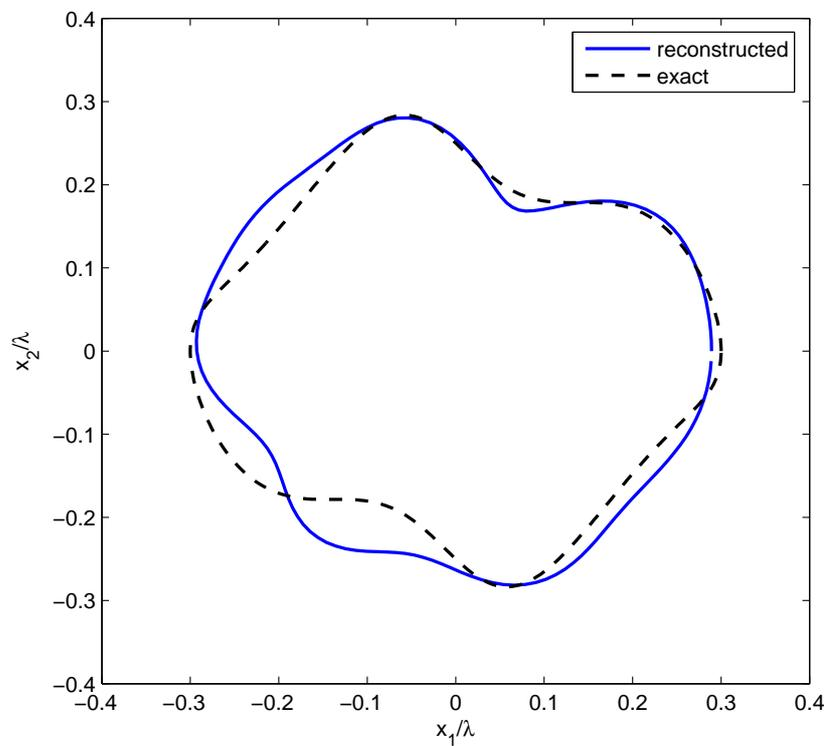
**Figure 5.11:** Exact and reconstructed geometries of a potato-shape object for  $\sigma = 0.1(S.m^{-1})$
