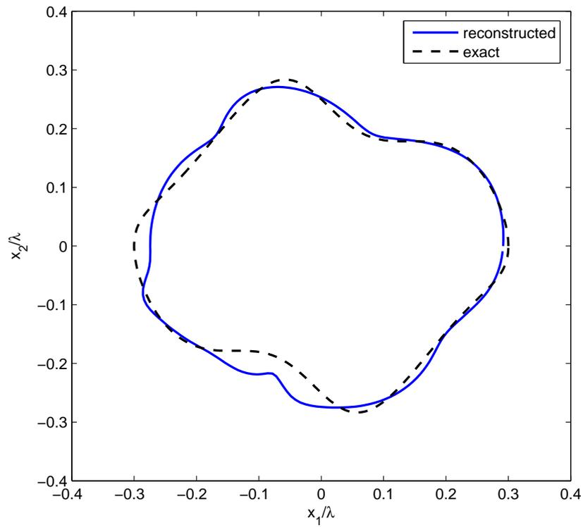
**Figure 5.10:** Exact and reconstructed geometries of a potato-shape object for  $\sigma = 0.01(S.m^{-1})$
