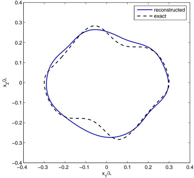
**Figure 5.3:** Exact and reconstructed geometries of a potato-shape object for  $\epsilon_r = 8$ . Noise-free case.
