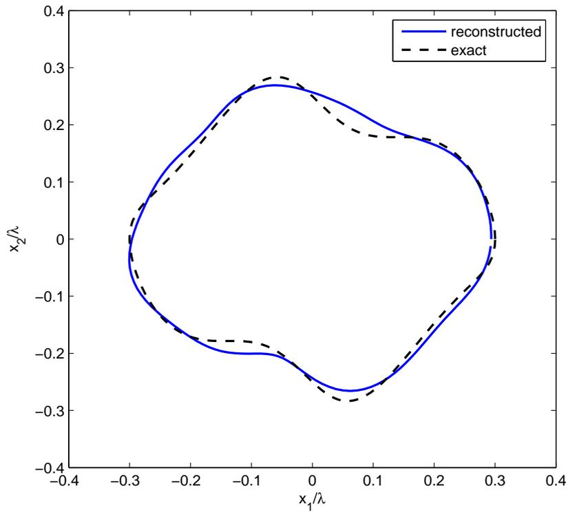
**Figure 5.7:** Exact and reconstructed geometries of a potato-shape object for the radius of the  $\beta$  is 10% greater than  $f_{max}$
