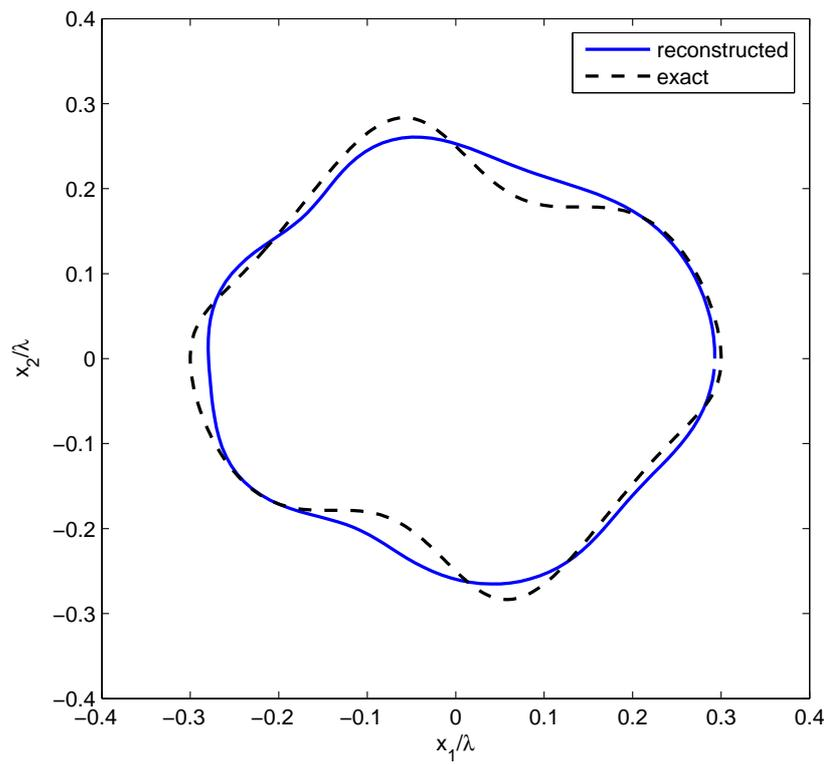
**Figure 5.13:** Exact and reconstructed geometries for single illumination
