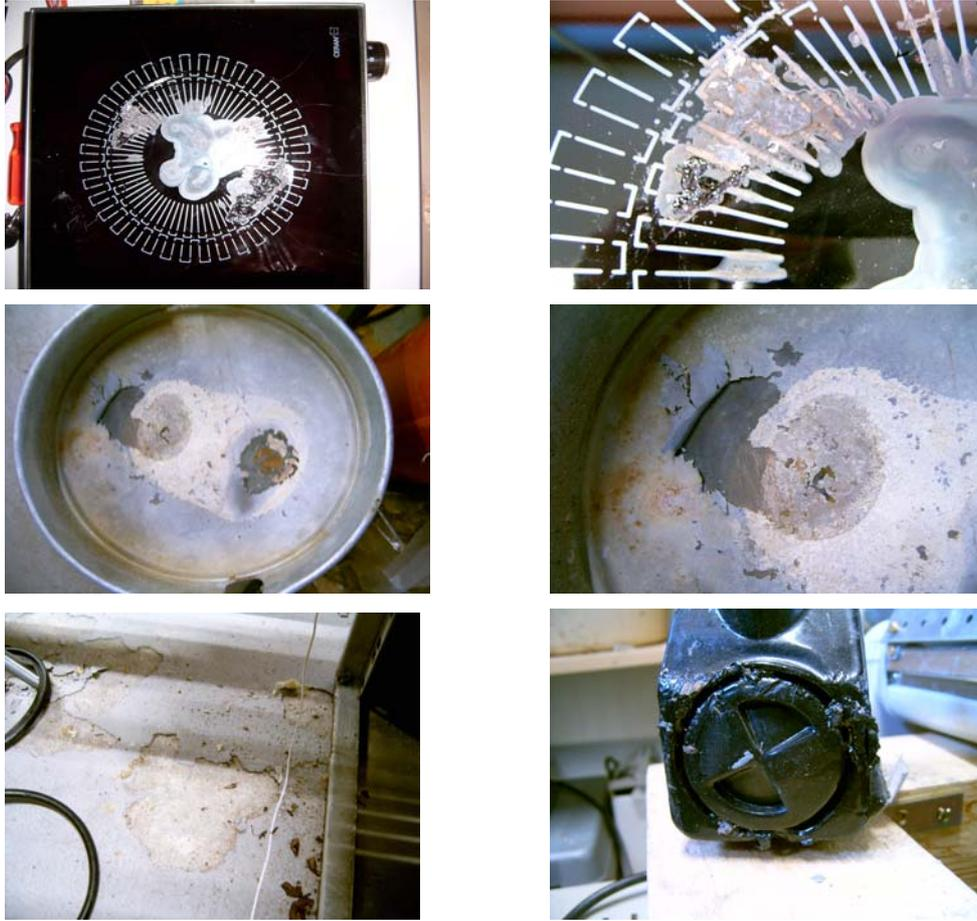
**Figure 4.21:** Effects of Benzyl alcohol onto the materials.
