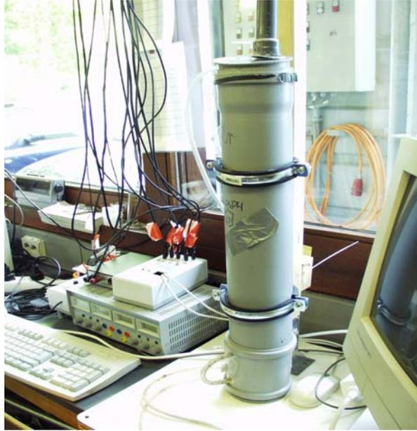
**Figure 3.1:** A view of biofilter reactor.
