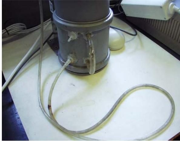
**Figure 3.3:** Water levelling pipe, Water sampling outlet, Air entrance hole.
