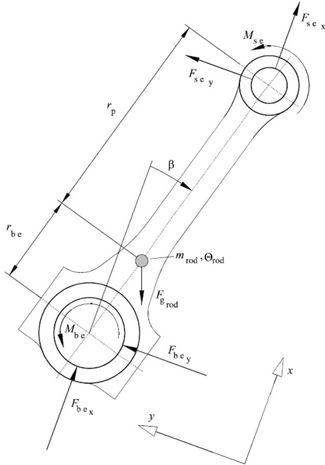
**Figure 3.3:** Free Body Diagram of Connecting Rod
