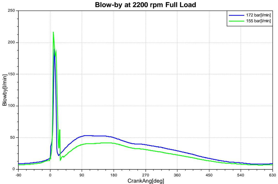
**Figure 6.31:** Blow-by at 2200 rpm Full Load
