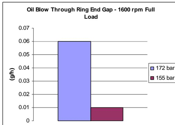
**Figure 6.3:** Oil Blow through Ring End Gap
