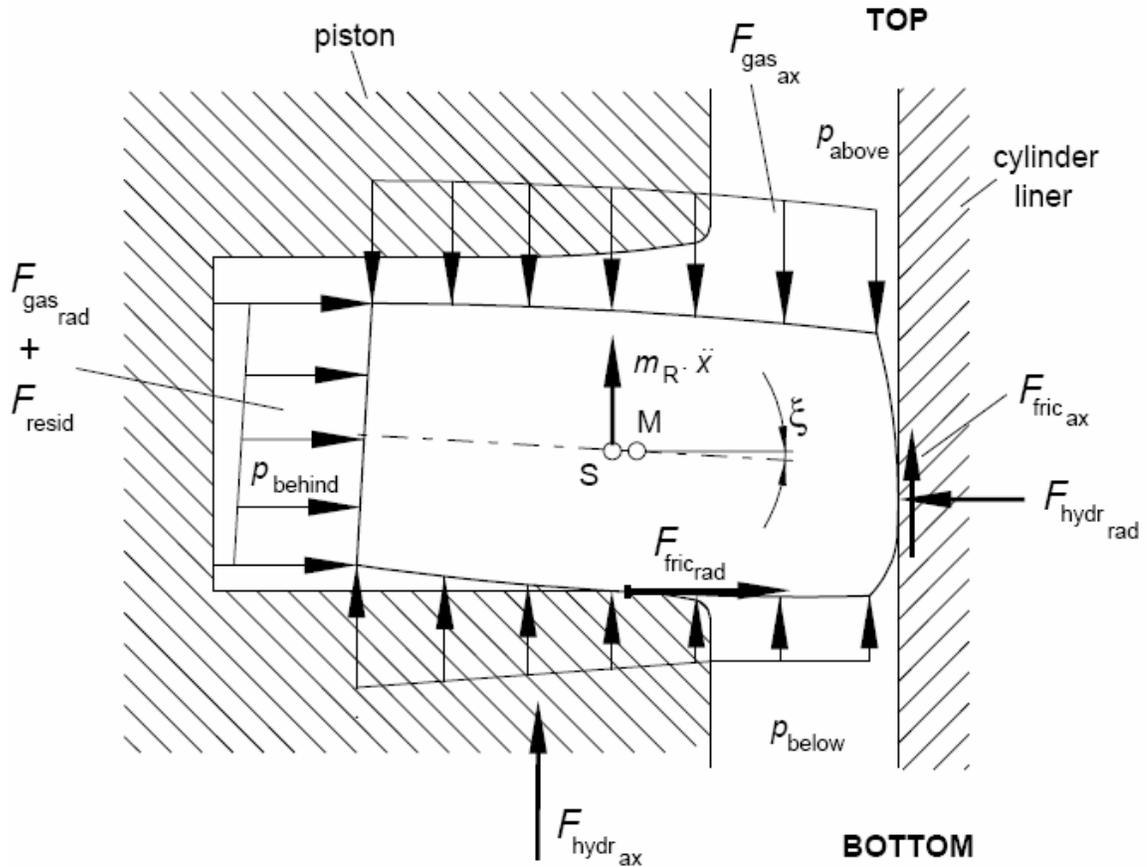
**Figure 2.7:** Forces Acting on a Piston Ring
