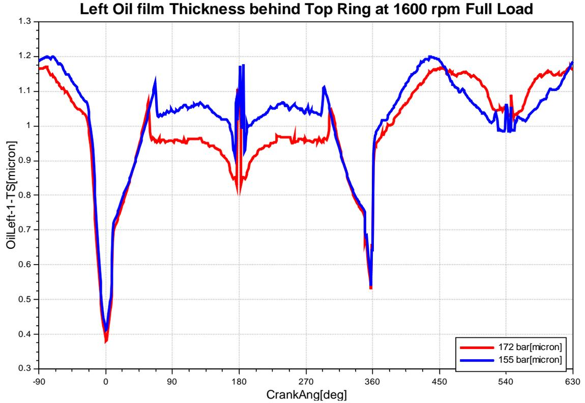
**Figure 6.15:** Left Oil Film Thickness behind Top Ring for 1600 rpm Full Load
