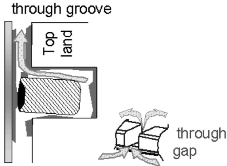
**Figure 2.2:** Oil Consumption by Reverse Gas Flow
