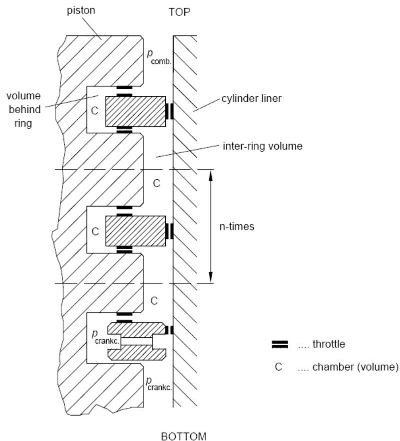
**Figure 3.6:** Gas Flow Model for Entire Ring Package
