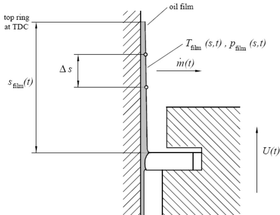
**Figure 3.13:** Oil Mass Flux into Combustion Gas
