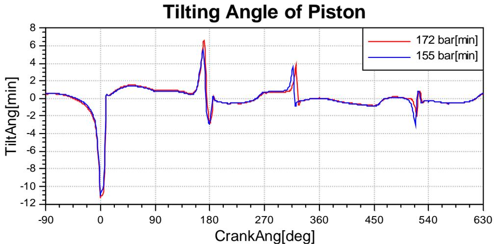
**Figure 6.7:** Tilting Angle of Piston
