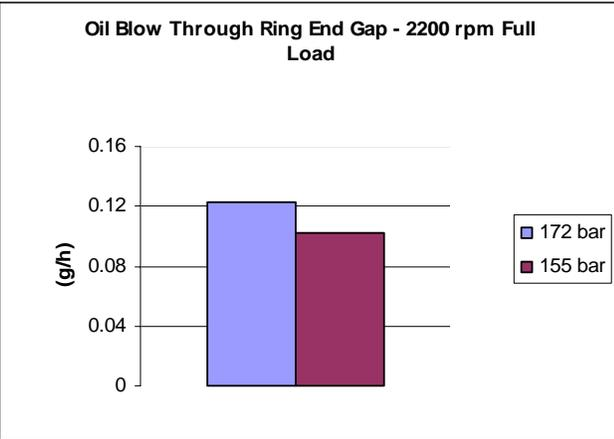
Figure 6.19: Oil Blow through Ring End Gap
