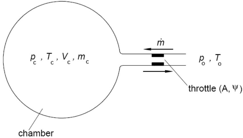
**Figure 3.7:** Gas Exchange Process from a Chamber
