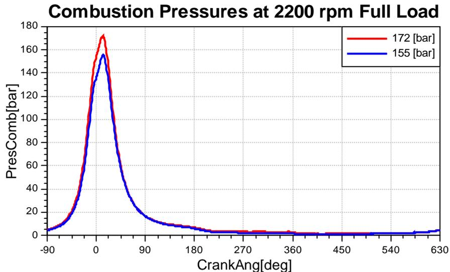
**Figure 6.17:** Combustion Pressure Variants at 2200 rpm Full Load
