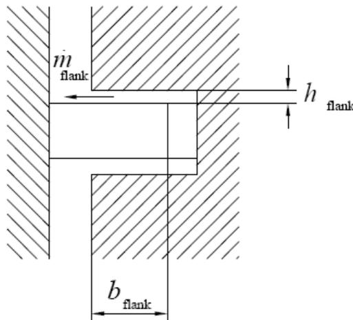
**Figure 3.15:** Oil Transport through Ring Groove
