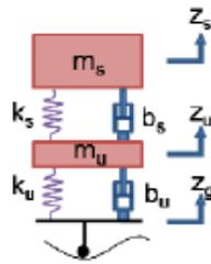
**Figure 1.4:** 2 DOF Quarter Car Suspension Model [8]
