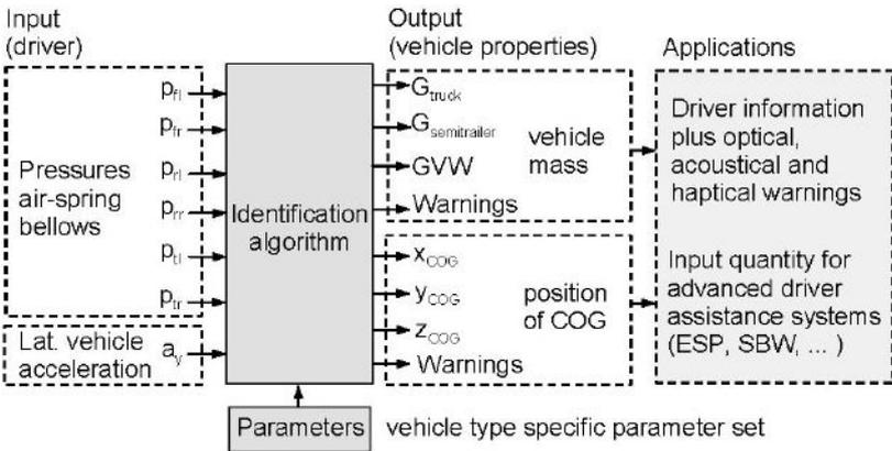
**Figure 1.3:** Payload Parameter Identification [7]
