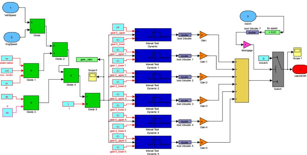
**Figure 4.15:** Enhanced Gear Estimation Algorithm
