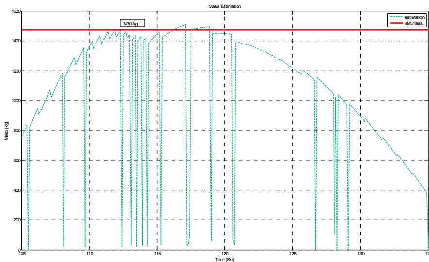
Figure 4.9: First Gear Acceleration Mass Estimation Results
