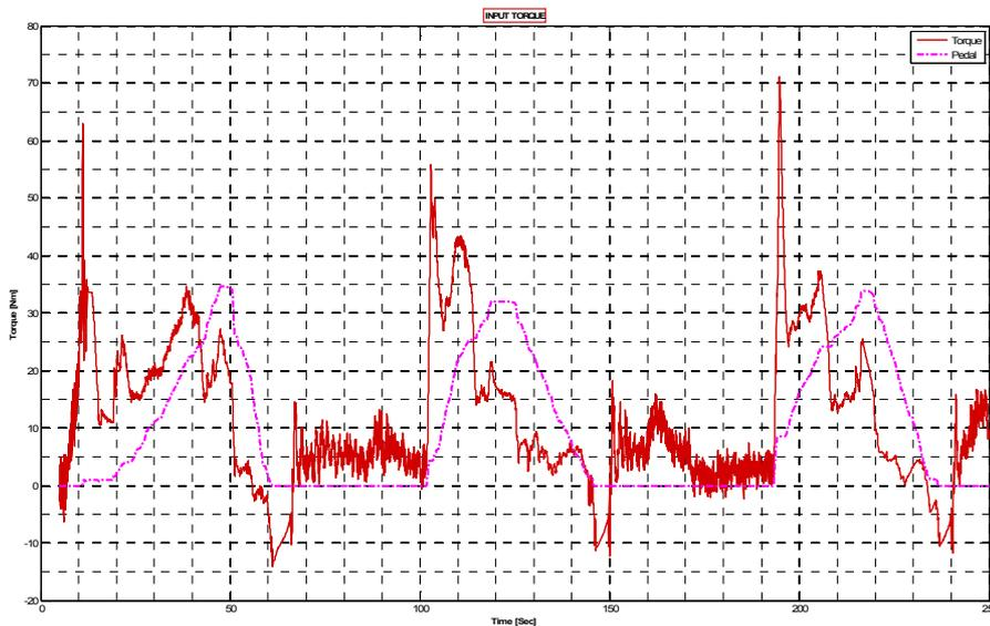
**Figure 4.6:** First Gear Torque Produced
