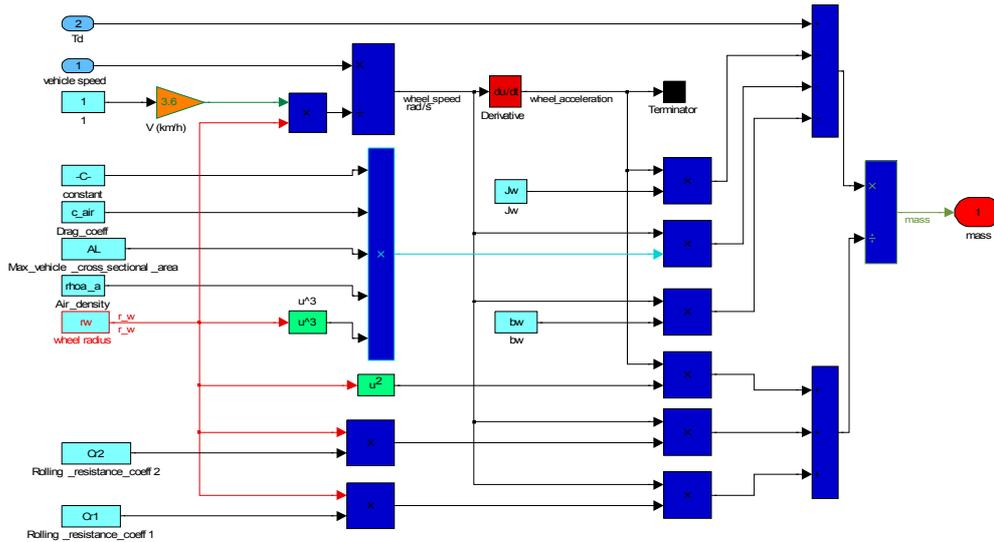
Figure 4.8: Mass Estimation Simulink Diagram
