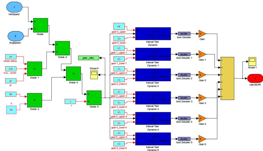
**Figure 4.13:** Initial Gear Estimation Algorithm Simulink Block
