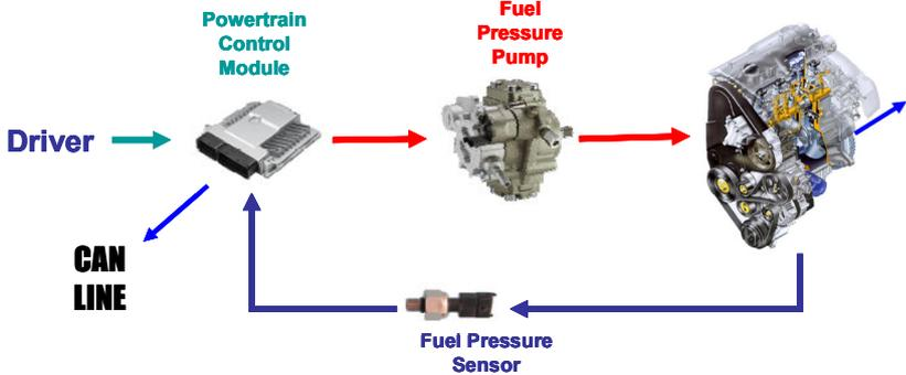
**Figure 4.1:** Engine System CAN Line
