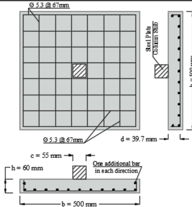
Figure 1. Slab geometry and reinforcement bars' details.
