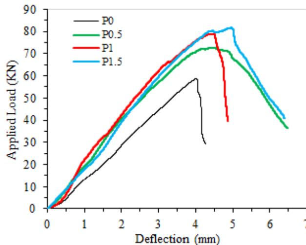
Figure 4. Load-Deflection curves for tested slabs
