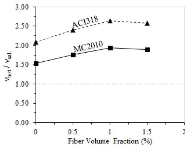
Figure 3. Comparison between tested shear stress and stresses proposed by MC2010 [5] and ACI318 [6]
