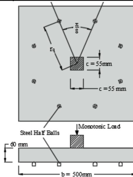
Figure 2. Test configuration
