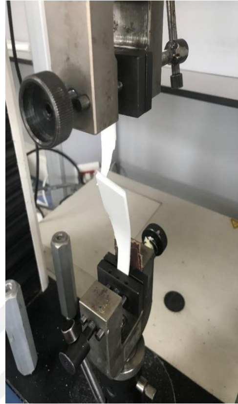
Figure 4. 45 PU2 Sample at initial stage and after rupture.
