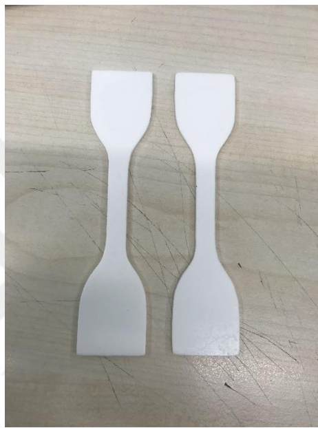
Figure 4. 37 Tensile test sample.
