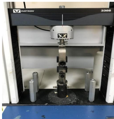
Figure 3. 4 Tensile strength and tear resistance analysis device.
