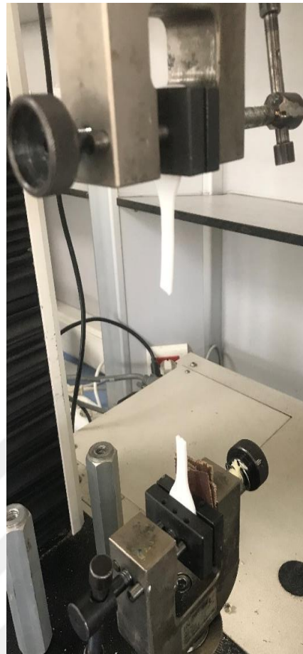
Figure 4. 39 PU2 sample during elongation and after breakage.
