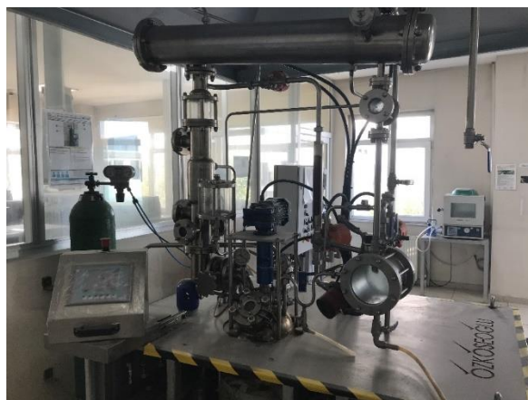
Figure 3. 9 Polyester polyol reactor.
