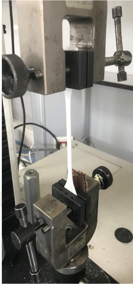
Figure 4. 39 PU2 sample during elongation and after breakage.
