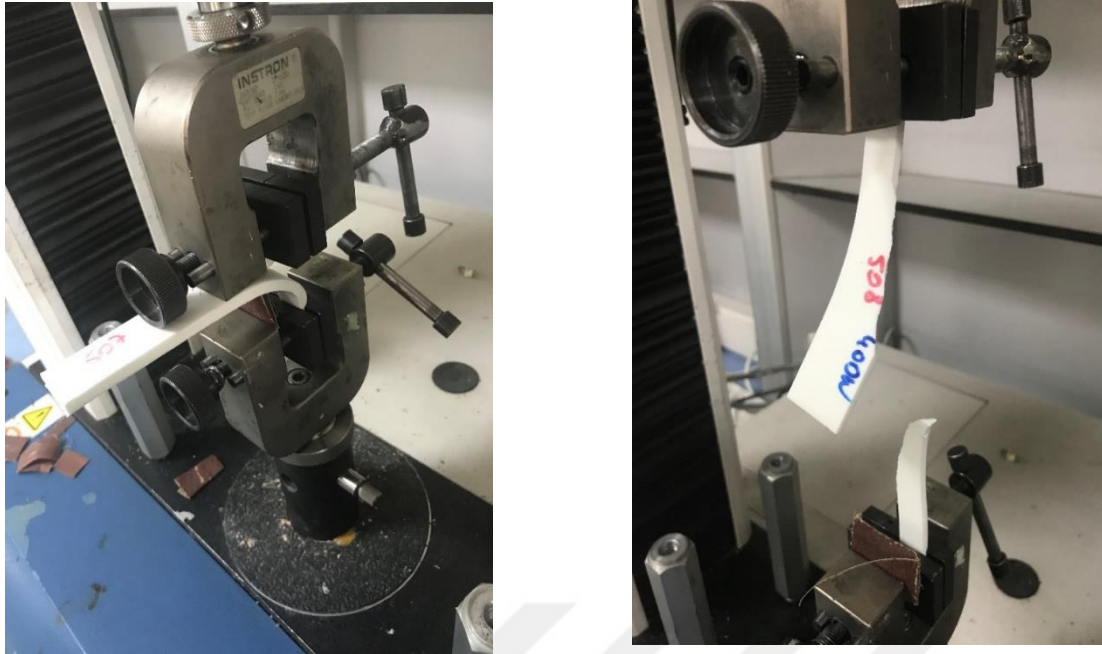
Figure 4. 47 PU4 Sample at initial stage and after rupture.
