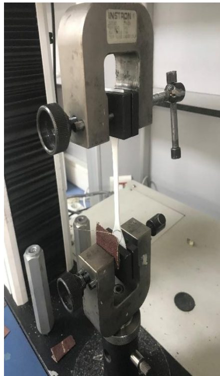
Figure 4. 40 PU3 sample during elongation and after breakage.
