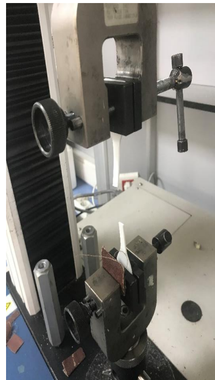
Figure 4. 40 PU3 sample during elongation and after breakage.
