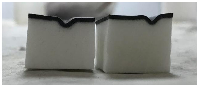
Figure 4. 33 Compression set samples.
