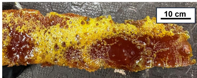
Figure 2.6 : Porosity in phenolic resin caused by gas release during curing.
