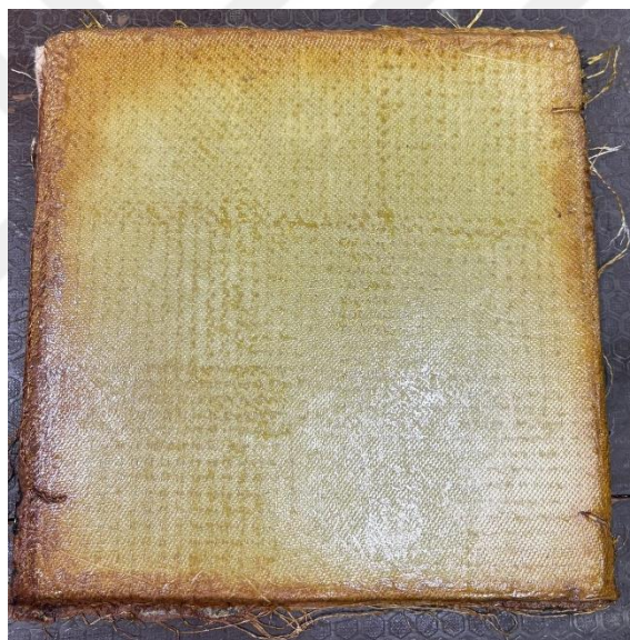
Figure 2.12 : Fully cured needle-punched composite plate obtained after stepwise curing profiling.
