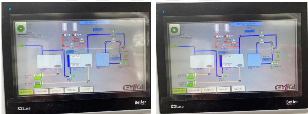
Figure 2.8 : The SCADA screen of the pilot scale IFAS MBR.
