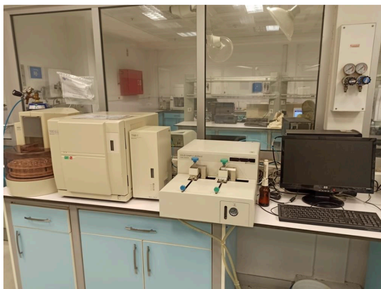
Figure 2.21 : Shimadzu TOC-VCPN Total Nitrogen-Total Organic Carbon Analyzer
