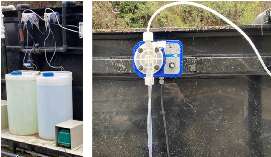
Figure 2.18 : The chemical tanks and chemical dosing pumps of the pilot scale IFAS MBR system.
