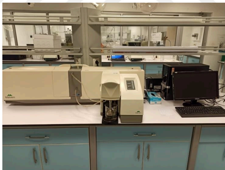
Figure 2.23 : Malvern Instruments Hydro 200 MU Mastersizer 2000 Device
