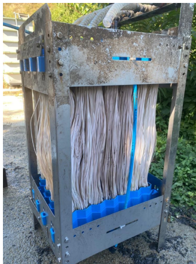
Figure 2.19 : The GEN MBR membranes used in pilot scale IFAS MBR system
