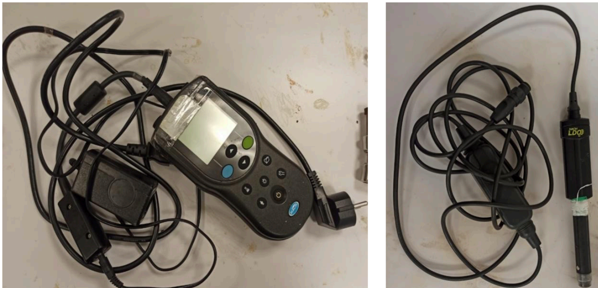
Figure 2.25 : The multi parameter measurement device and dissolved oxygen probe
