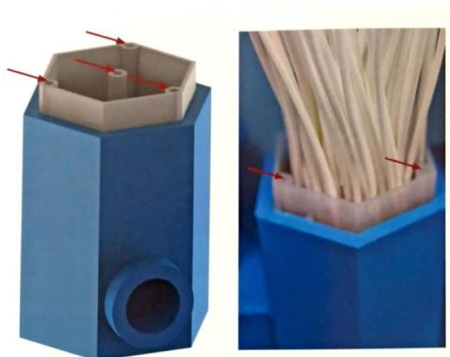
Figure 2.12 : The membrane aeration of the pilot scale IFAS MBR system.
