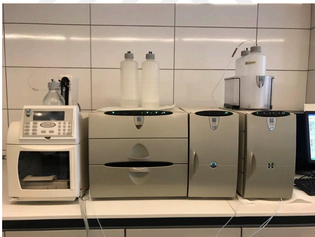
Figure 2.22 : Dionex ICS 300 ion chromatography (IC).
