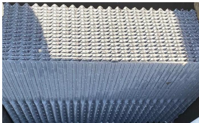
Figure 2.20 : The carrier material used in the pilot-scale IFAS MBR system.
