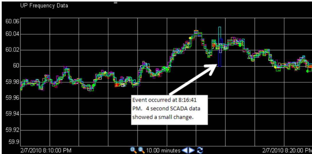
Figure 1.2 : Change in frequency captured by SCADA [3]
