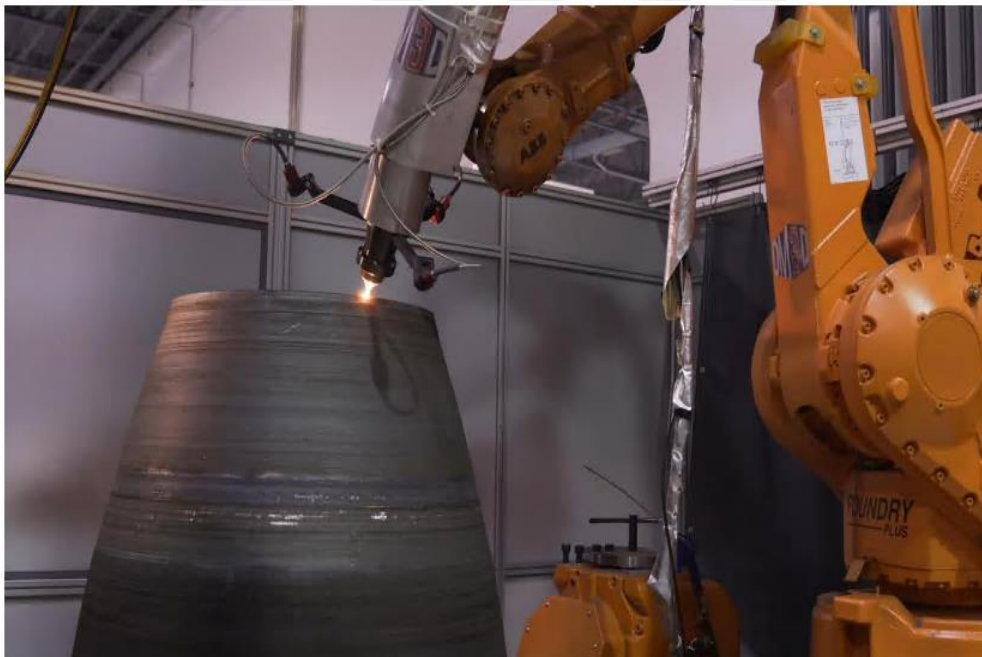
Figure 2.2 : Production of a large part by DED method [26].
