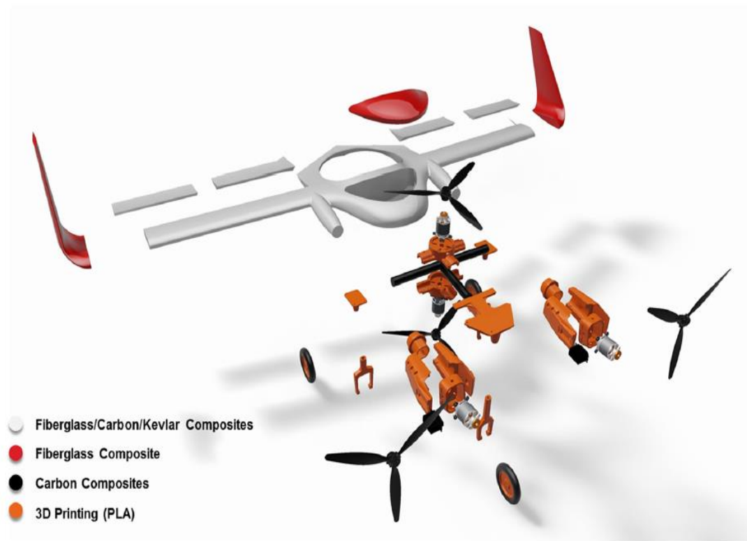
Figure 1.6 : The parts of unmanned aerial vehicles [21].
