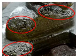
Figure 1.5 : Surface after infiltration of the slurry [17].
