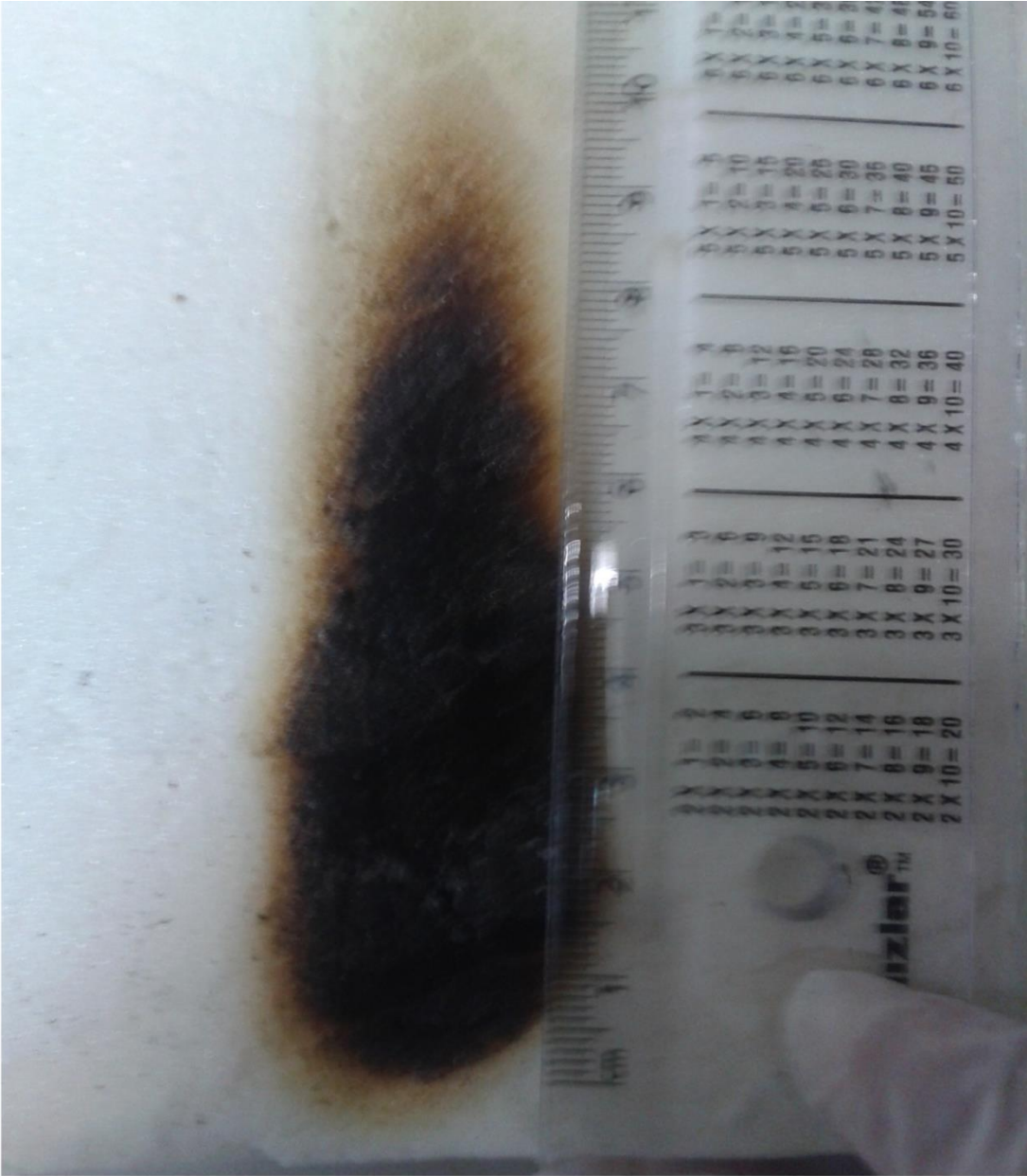
Figure A.10 : THEIC-TCPP (FR-2 20 % in polymix) at polyurethane rigid foam (8 cm)
