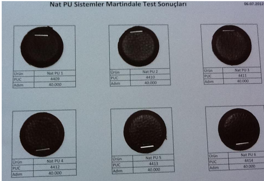
Figure 4.91 : Abrasion Test Results (Martindale at Leather).
