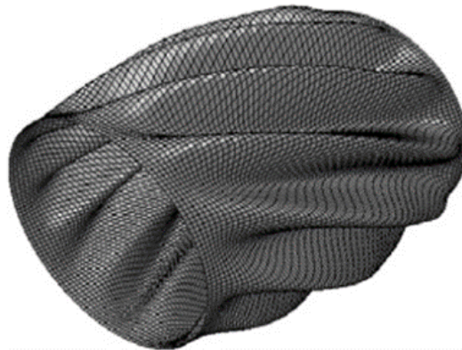
Figure 4.1 : Linear buckling reference source analysis result [6].
