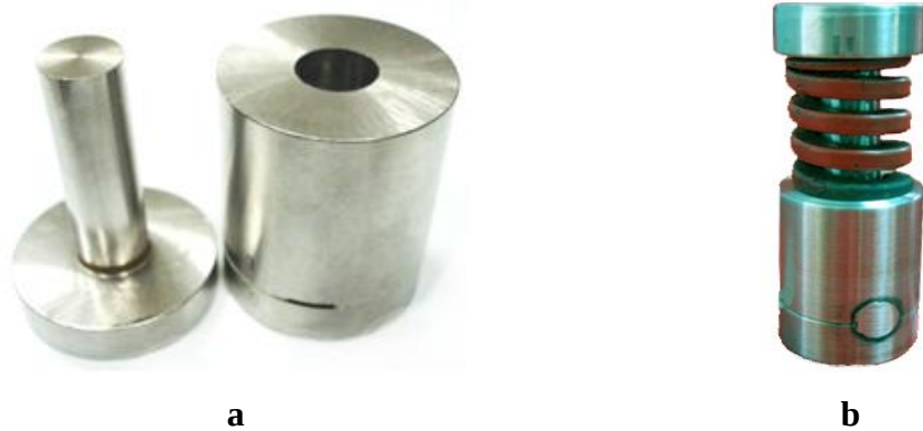
Figure 3.3 : a) Primarily designed b) Spring added tape extrusion mold.
