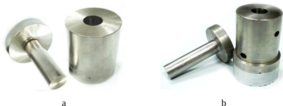
Figure 3.6 : a) Block body b) Modular body wire extrusion mold.
