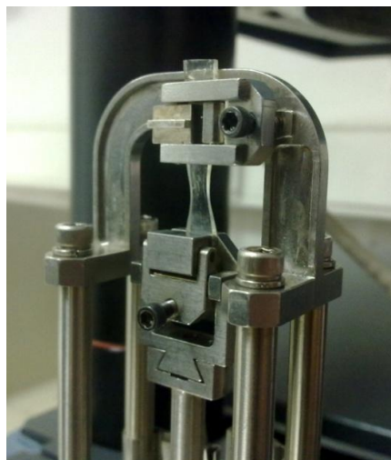
Figure 4.19 : Tape sample view during DMA measurement.
