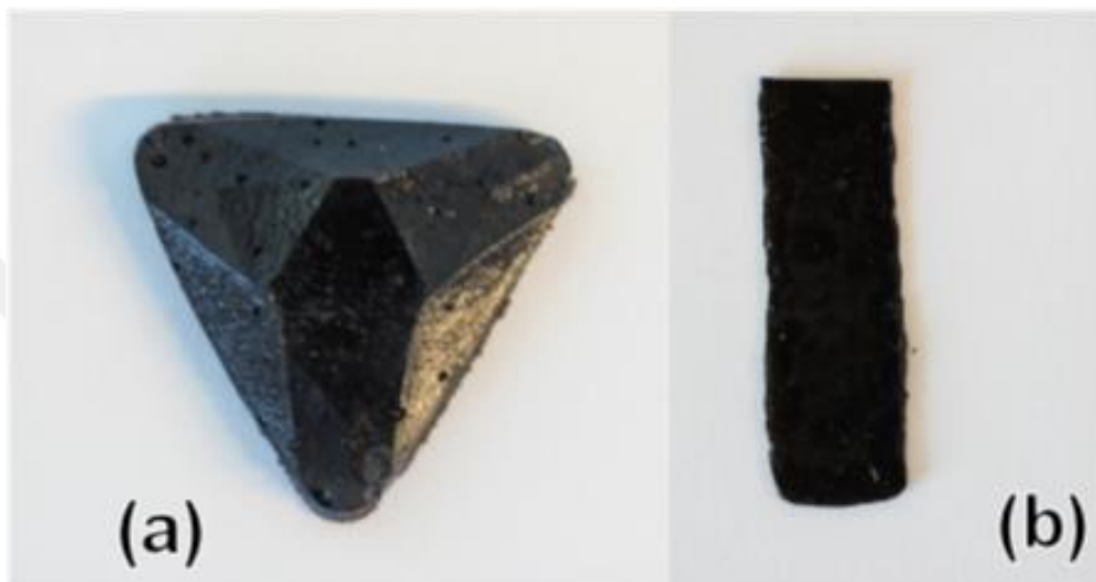
Figure 4.5 : Images of poly(Va-Bz 40 -S 20 -ionone 40 ) as mold (a) and film (b).
