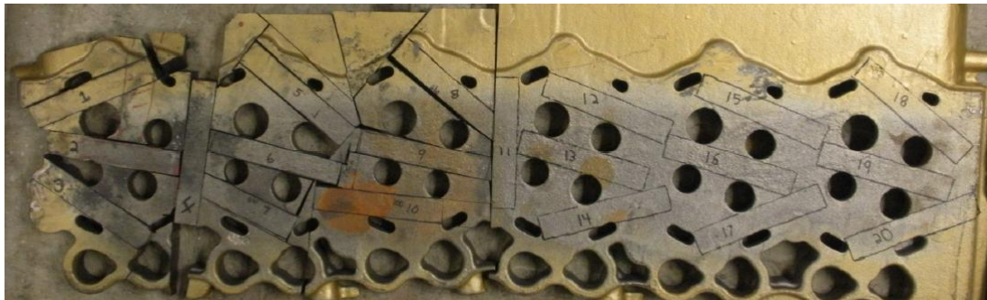
Figure 7.6 : Specimens of CGI450 material from cylinder head.
