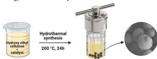
Figure 1. Schematic representation of one pot CS synthesis procedure.
