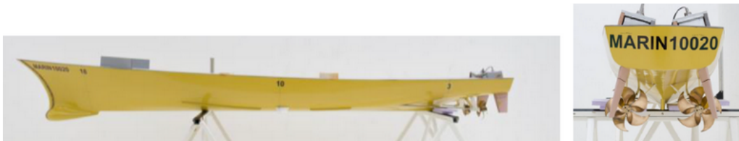
Figure 1.1 : A scaled down model of 5415M built by MARIN.
