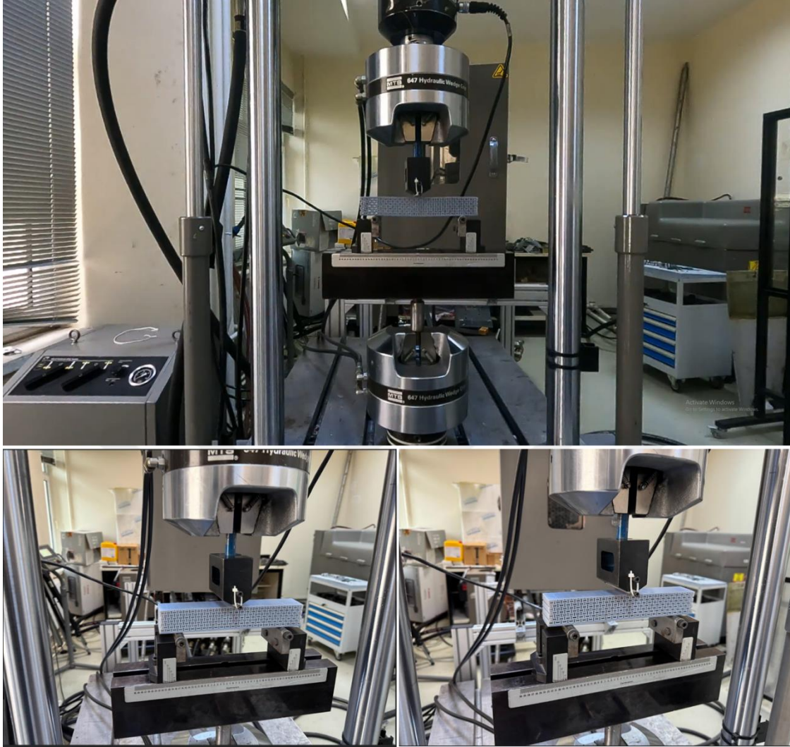
Figure 2.112: 3-Point Bending Test Setup for Anti-tetrachiral Structure.
