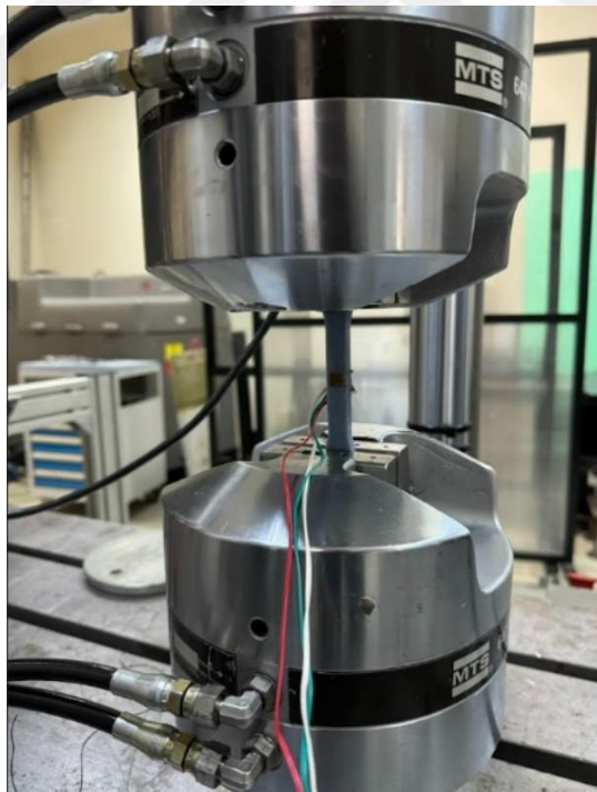
Figure 2.20: Tensile test setup for the second specimen.
