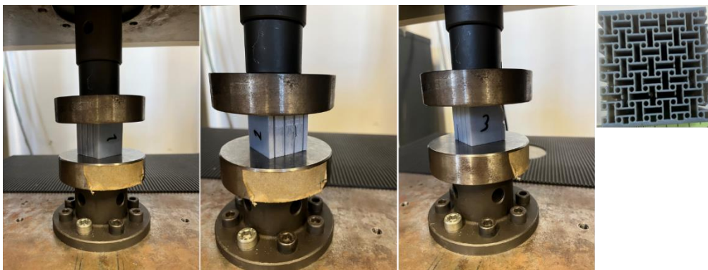
Figure 2.32: Cubic specimens of anti-tetrachiral structure used in the compression test.
