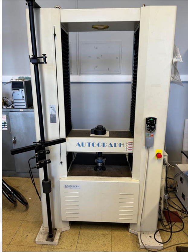
Figure 2.33: Shimadzu Autograph AG-IS 50 kN universal testing machine.
