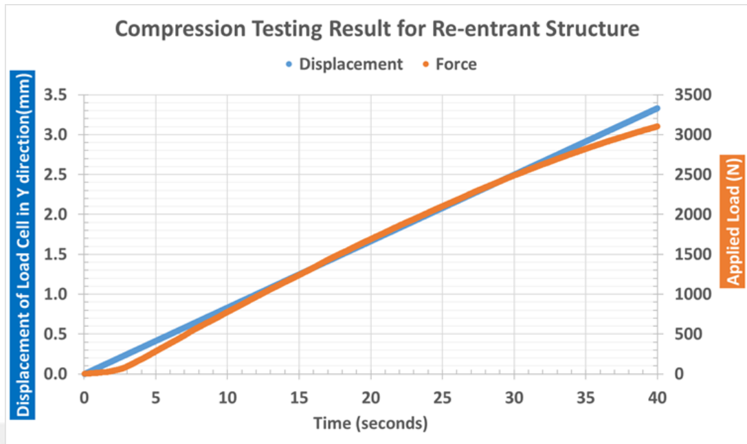
Figure 2.123: Experimental load–displacement versus time curve of the re-entrant structure under compression.
