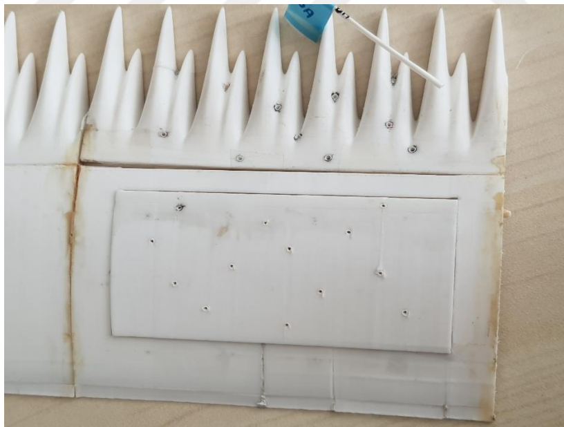
Figure 3.3 : Pressure taps on wing .
