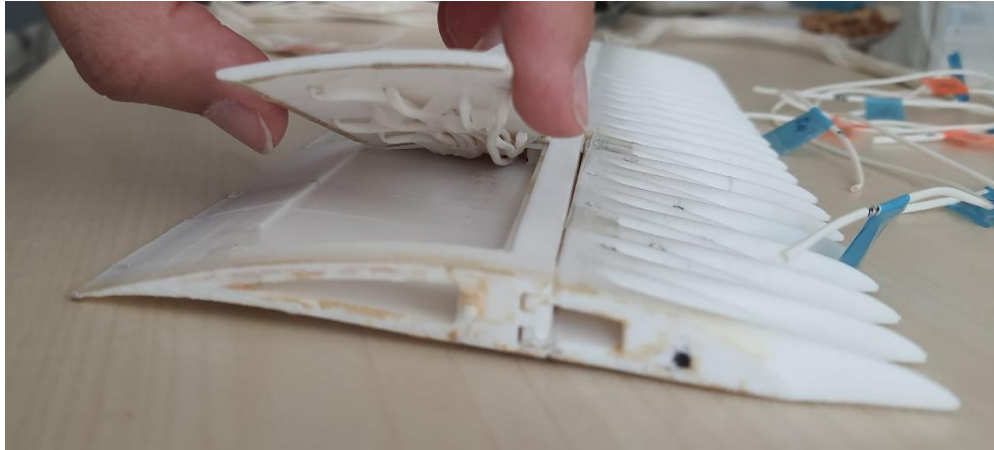
Figure 3.4 : Inserted hoses and cover of rear part of the wing.
