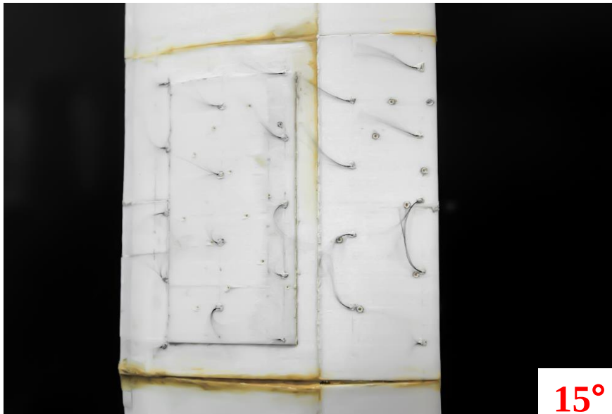
Figure 4.6 : FV of baseline wing at 15° AoA.
