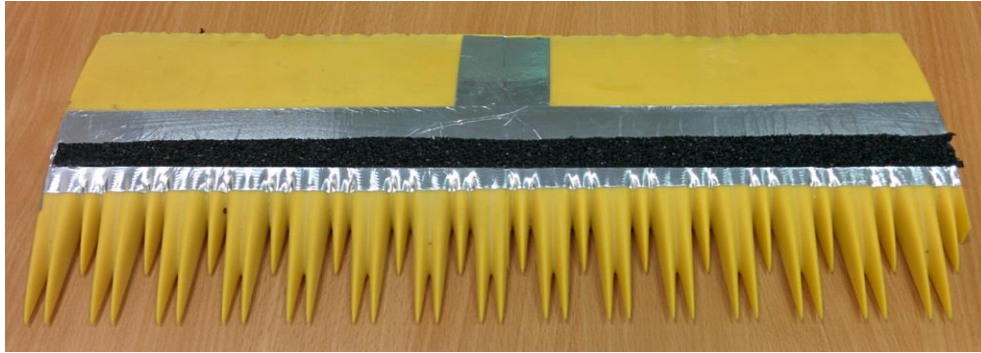
Figure 1.8 : 3D DW design used in the study of Chaitanya et al [72].
