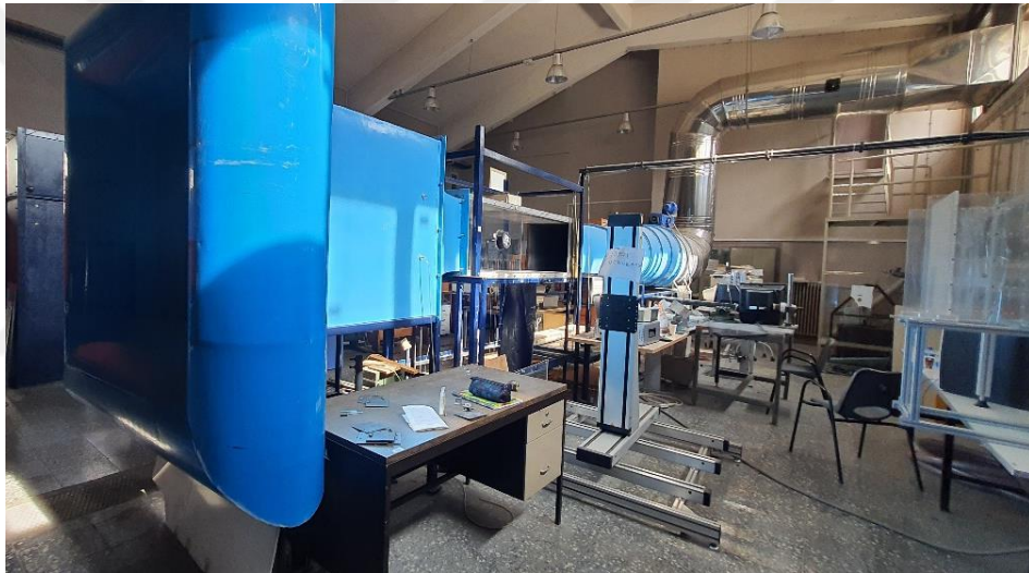
Figure 3.1 : Open circuit, subsonic, 50 x 50 cm wind tunnel.
