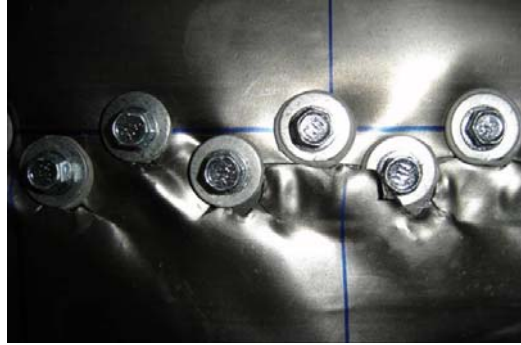
Figure 7.26: Infill Tear in Upper North Corner (Specimen SW-A-H, Cycle 32 and Top Disp. of -50.39mm)
