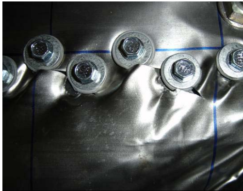
Figure 7.25: Infill Tear in Upper North Corner (Specimen SW-A-H, Cycle 32 and Top Disp. of +50.39mm)
