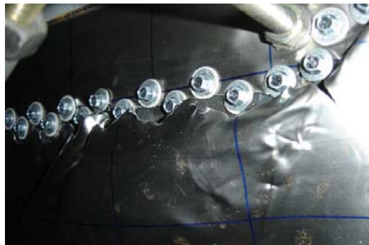
Figure 7.27: Propagation of Infill Tear in Upper North Corner (Specimen SW-A-H, Cycle 33 and Top Disp. of +50.39mm)
