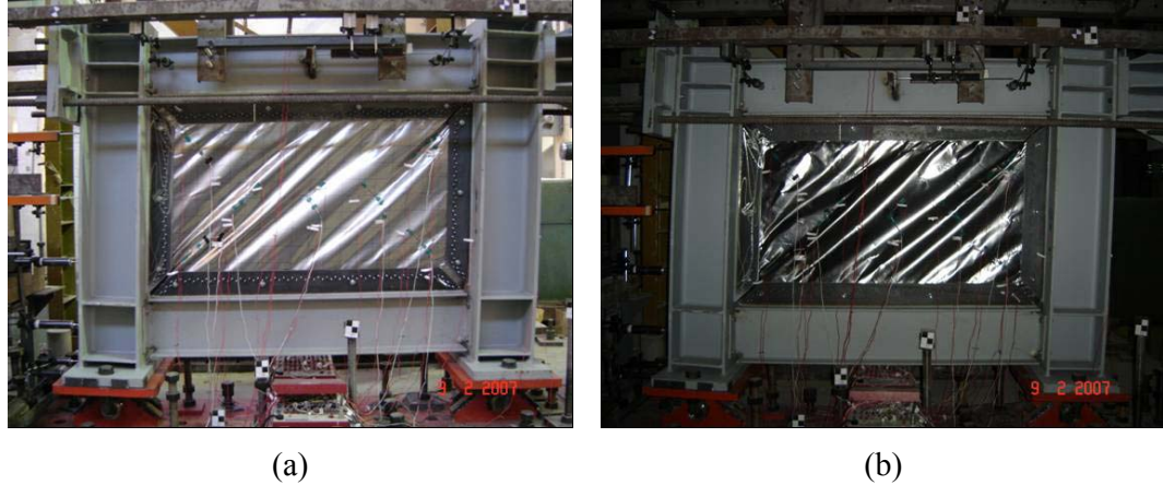
Figure 7.29: (a) Buckling of Infill at -6\delta_y in Cycle 32 and (b) Buckling of Infill at -6\delta_y in Cycle 33 (Specimen SW-A-H, Cycle 32 and Cycle 33 Top Disp. of -50.39\text{mm} )
