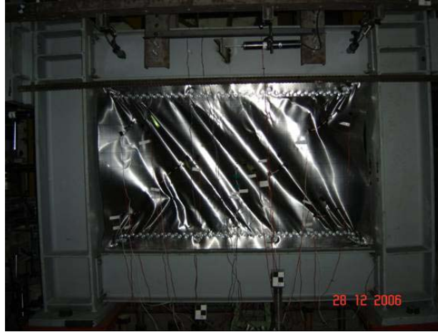
Figure 7.48: Infill Plate Buckling Waves Configuration (Specimen SW-B-H, Cycle 34 and Top Disp. of +32.40mm)
