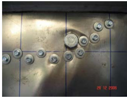
Figure 7.37: Plastic Folds in Upper South Corners (Specimen SW-B-H, Cycle 13 and Top Disp. of -4.48mm)
