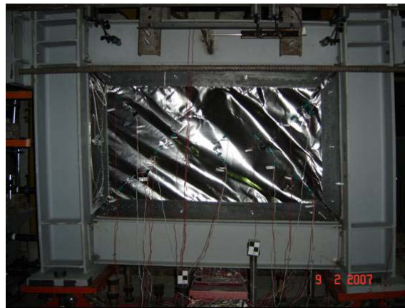
Figure 7.30: Buckling of Infill Plate (Specimen SW-A-H, Cycle 34 and Top Disp. of +58.80\text{mm} )
