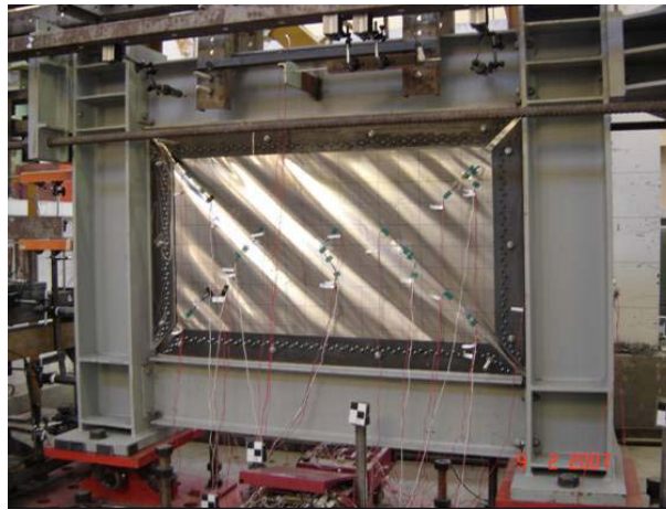
Figure 7.18: Infill Plate Buckling (Specimen SW-A-H, Cycle 25 and Top Disp. of +25.19mm)
