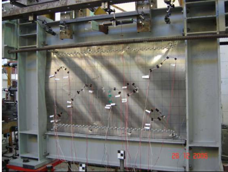
Figure 7.40: Infill Plate Buckling (Specimen SW-B-H, Cycle 22 and Top Disp. of +7.20mm)
