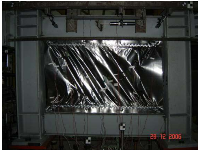
Figure 7.53: Infill Plate Buckling Waves Configuration (Specimen SW-B-H, Cycle 38 and Top Disp. of +50.61mm)
