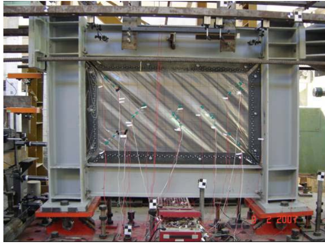
Figure 7.22: Infill Plate Buckling (Specimen SW-A-H, Cycle 30 and Top Disp. of +41.97mm)
