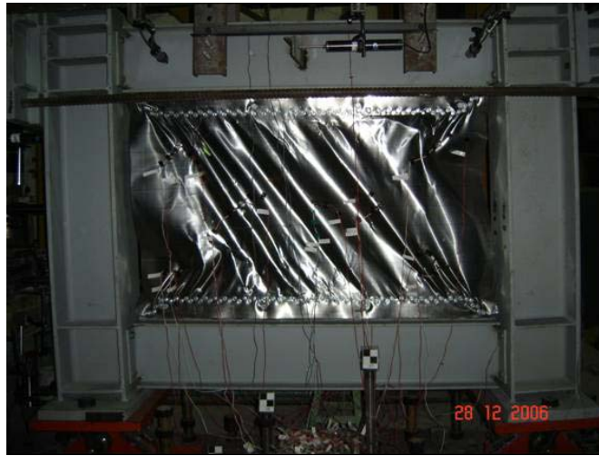
Figure 7.51: Infill Plate Buckling Waves Configuration (Specimen SW-B-H, Cycle 36 and Top Disp. of +40.51mm)
