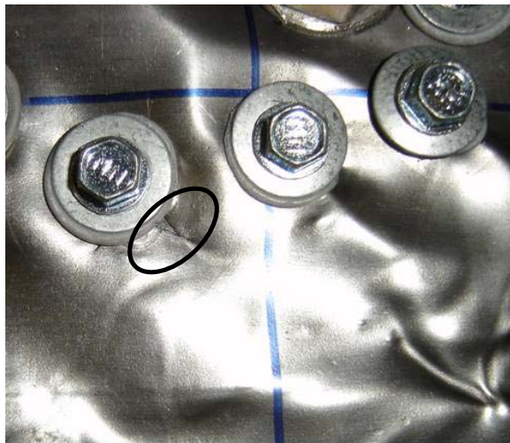
Figure 7.23: Infill Tear in Upper North Corner (Specimen SW-A-H, Cycle 30 and Top Disp. of +41.97mm)
