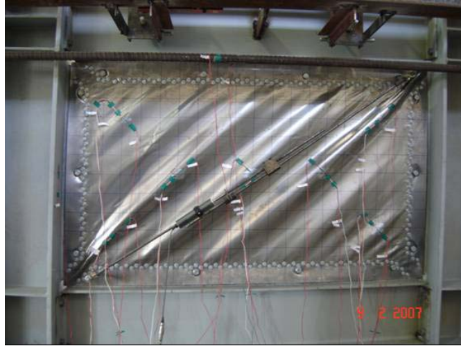
Figure 7.20: Infill Plate Buckling (Specimen SW-A-H, Cycle 28 and Top Disp. of +33.72mm)
