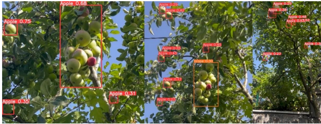
Figure 3.6 : Fruit detection model real-world results (apple)
