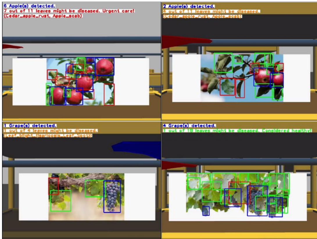
Figure 3.12 : Annotated images from simulation
