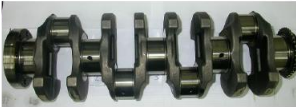
Figure 9.3 : Final shape of the cast crankshaft
