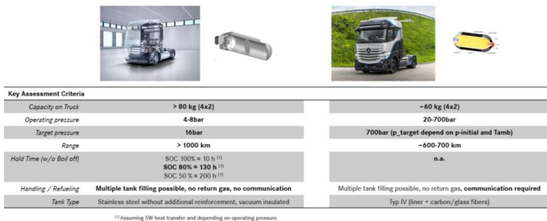
Figure 2.20: Comparison of two heavy duty trucks equipped with sLH 2 and CHG700 [16].
