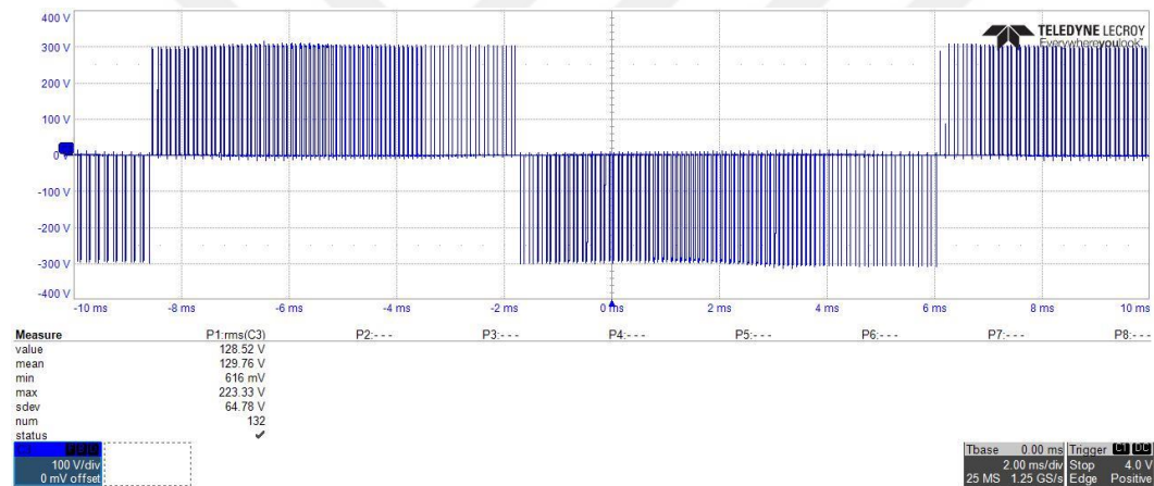
Figure 9.17: Phase to phase voltage of the motor @1300 rpm.
