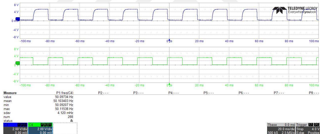
Figure 9.25: The input and the output signals of the optocoupler.
