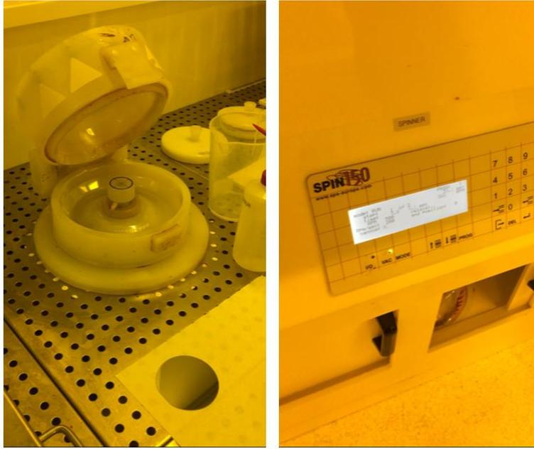
**Figure 3.1:** Spin Coater with the control panel.
