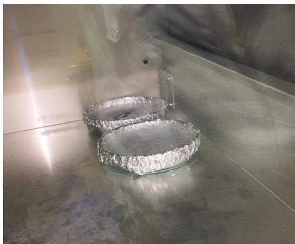
**Figure 3.6:** Degassing in the vacuum oven.
