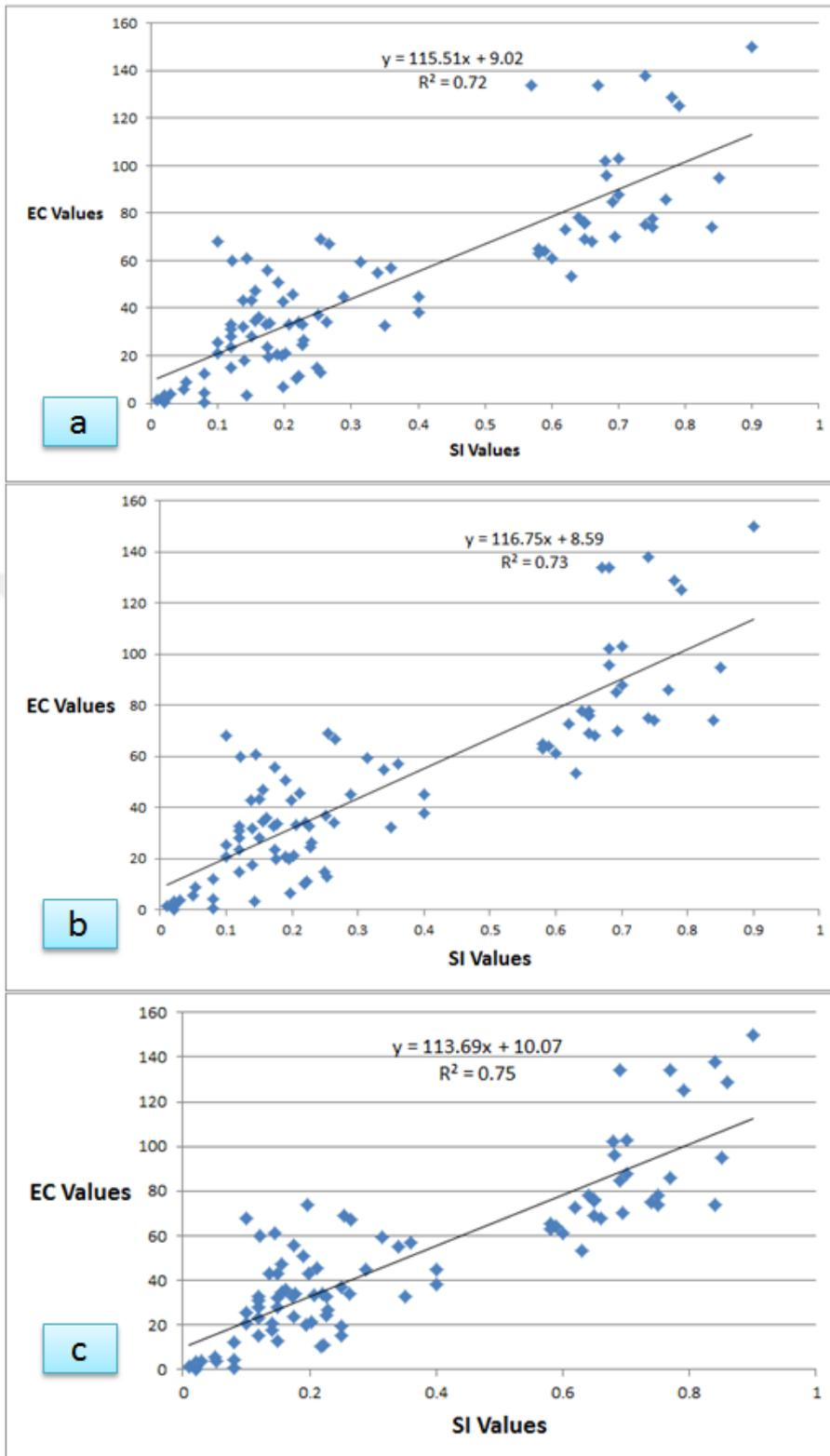
**Figure 5.3 :** Linear regression results between ground measurement EC values and SI values (a) SI1, (b) SI2, (c) new SI for Urmia Lake.
