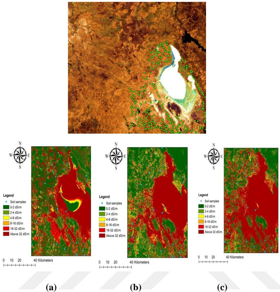
**Figure 5.6 :** Soil salinity maps generated by utilizing (a)- SI1, (b)- new generated soil salinity index, and (c)- SI2 index in Tuz Lake Basin.
