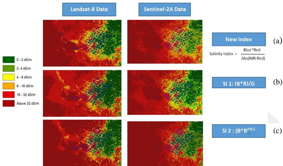
**Figure 5.4 :** Soil salinity maps generated by (a)-utilizing new generated soil salinity index, (b)-SI1 and (c)-SI2 derived from Landsat-8 OLI and Sentinel-2A data in the Bonab Region.
