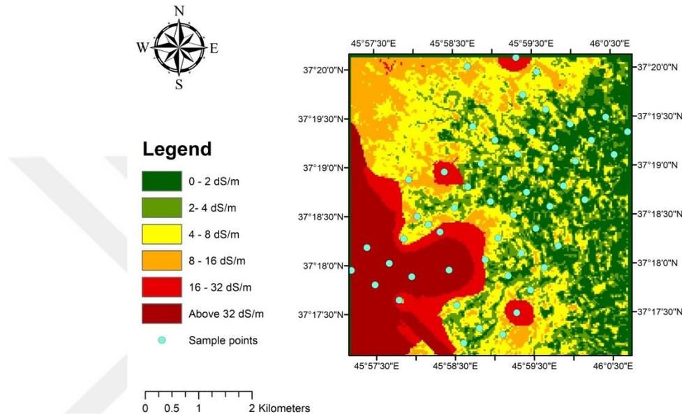
**Figure 5.9 :** Output map of Cubist model using 3 salinity indices and 4 ordinary kriging raster data including (Na, SAR, Ca, Mg) in the Bonab Region.
