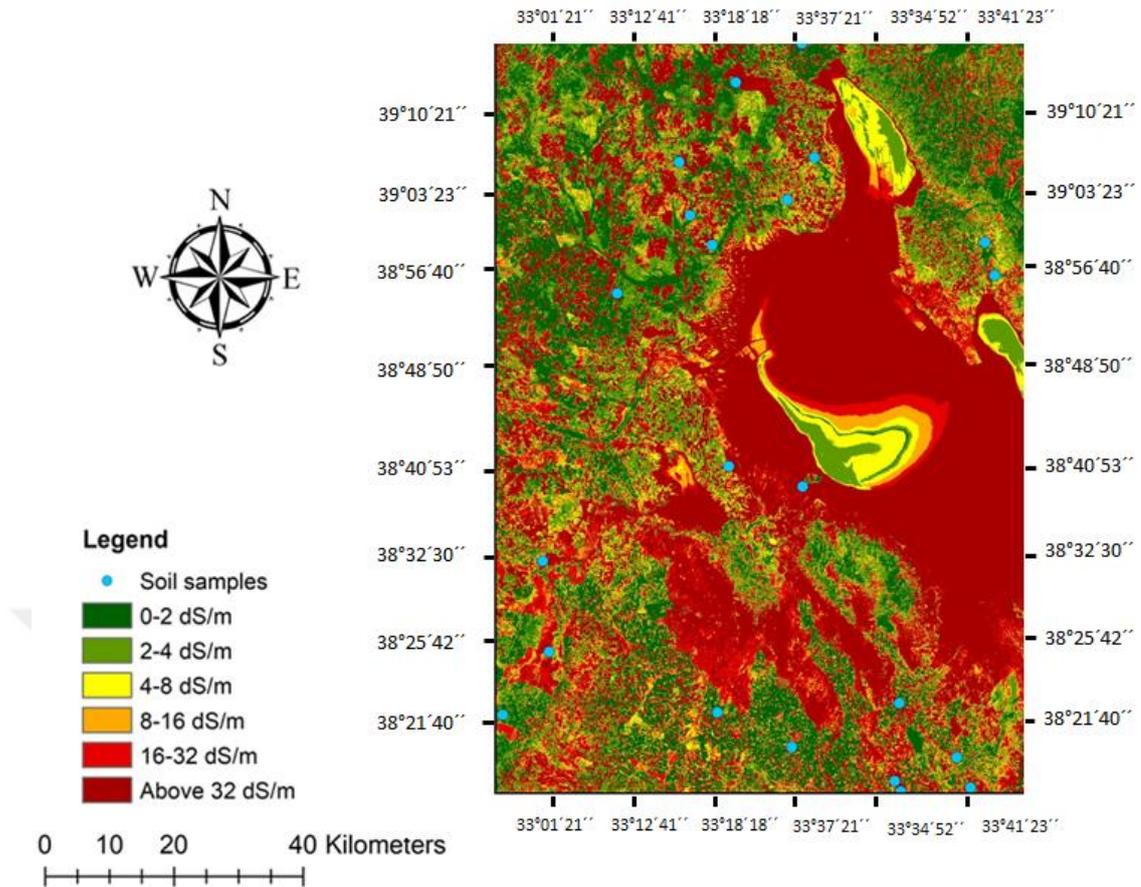
**Figure 5.19 :** Output map of Cubist model using 3 RS data and 3 ordinary kriging raster data in the Tuz Lake Basin.
