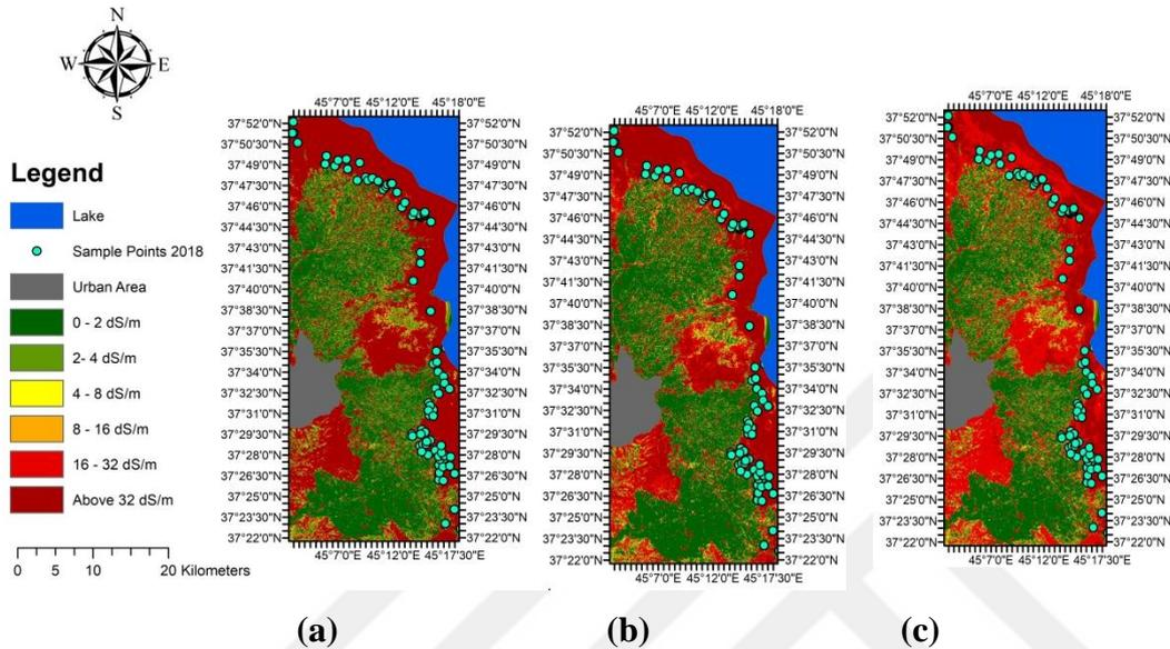
**Figure 5.5 :** Soil salinity maps generated by utilizing (a)- SI1, (b)- new generated soil salinity index, and (c)- SI2 index derived from Landsat-8 data in the West playas of Urmia Lake Basin.
