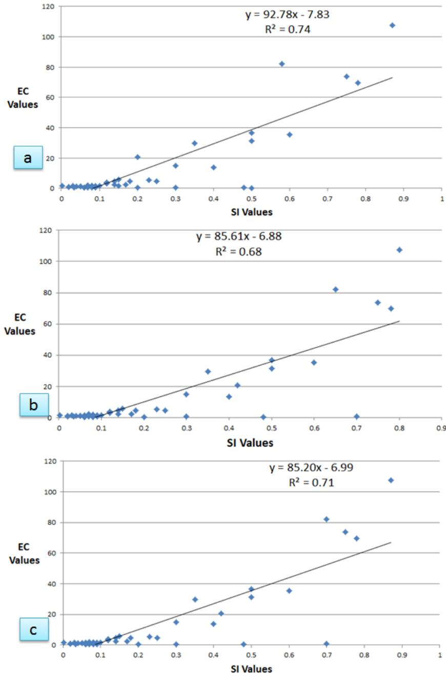
**Figure 5.1 :** Linear regression results between ground measurement EC values and SI values (a) new SI, (b) SI2, (c) SI1 for Bonab Region.
