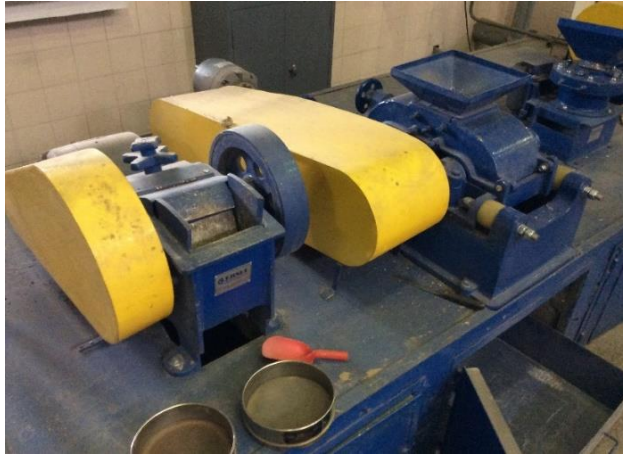
Figure 2.2: Rock crusher equipment.
