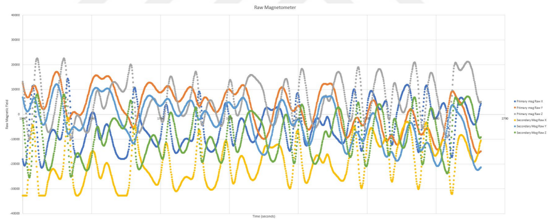
Figure 4.15: Raw magnetic field measurement data of deployable and redundant magnetometer collected by SharjahSat-1
