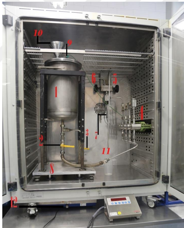
Figure 6.3 : Furnace with substance-carrying parts of the PGSS plant: (1) Vessel, (2) Ball valve, (3) Ball valve for cleaning, (4) Four pump heads of the four-head piston pump, (5 and 6) Three-way valve, (7) Pressure sensor, (8) The plate, (9) Thermo-element type K, (10) Funnel, (11) Bypass-pipe, (12) Balance.
