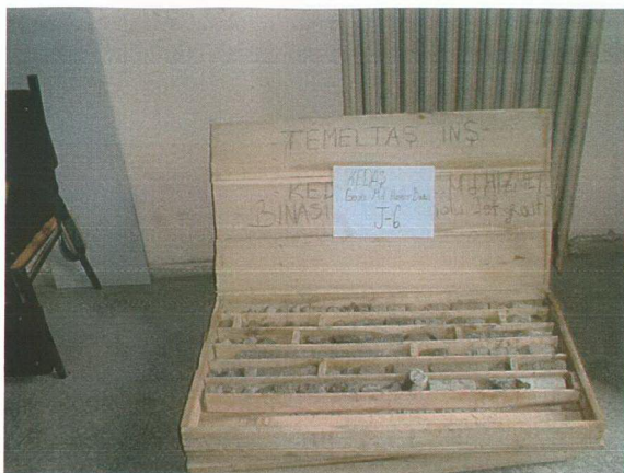
Fig. 3.20 Core Samples of Column J – 6
