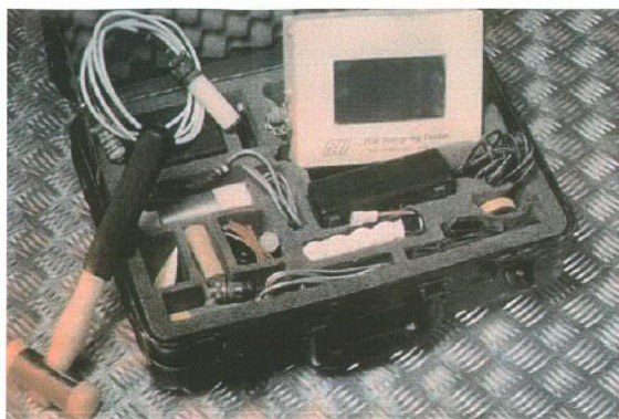
Fig. 2.22 Pile Integrity Testing Equipment
