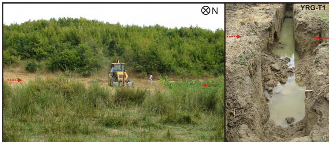
Figure 6.28 : View of the location of T1 at the eastern end of the basin. Red lines indicate the most-possible location of the fault zone. The presence of unconsolidated units and high ground-water level caused instability within the trench and walls collapsed when reached the fault zone.
