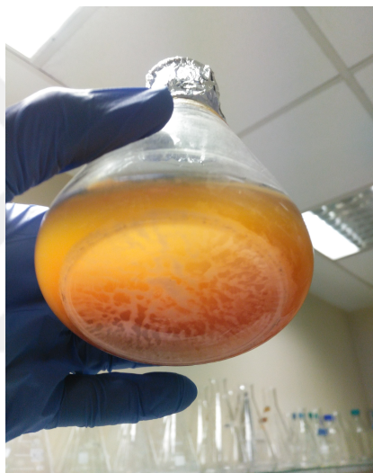
Fig. 3.4 : Addition of <0.5M urea+ \text{CaCl}_2 \cdot 2\text{H}_2\text{O} to the grown batch and observed precipitation.
