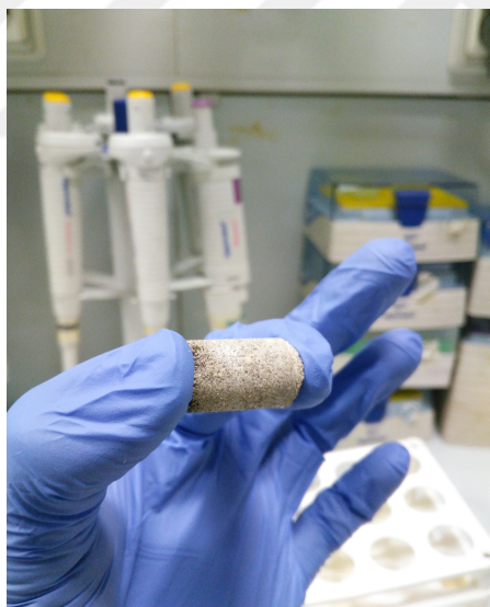
Fig. 3.11 : Successful cementation of a 5ml 200-150µm sized Olive Avantgarde sample.
