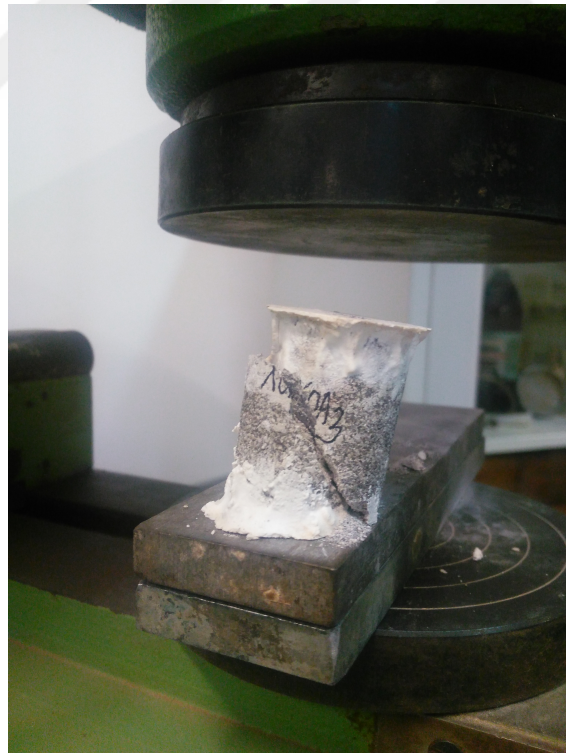
Fig. 3.31 : Deformation of sample no. XOA3 after the compression test.
