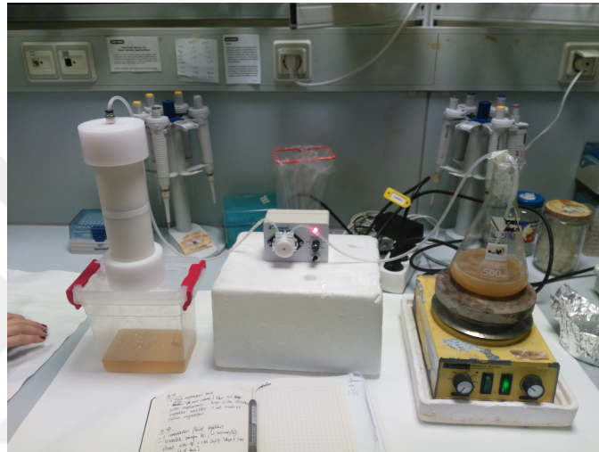
Fig. 3.12 : Calcite in situ precipitation system during cementation fluid injection intervals.
