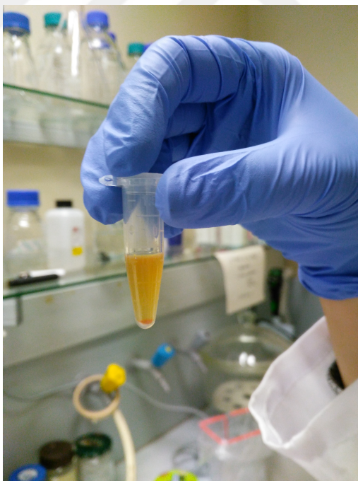
Fig. 3.3 : Observed color change and precipitation after the addition of Nessler's reagent.
