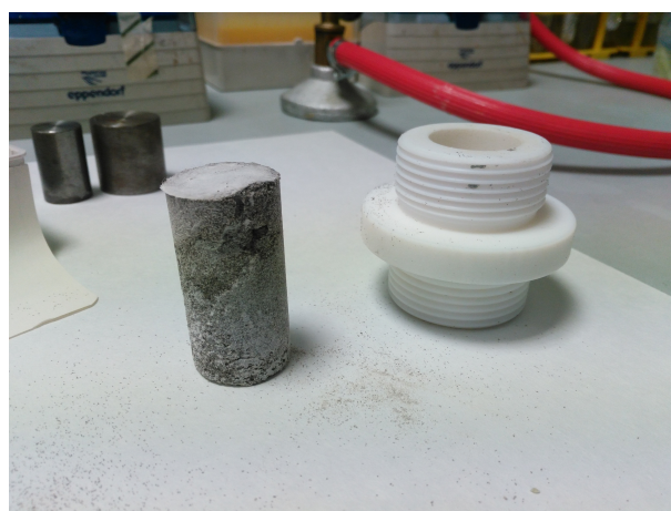
Fig. 3.13 :250-500µm sized Olive A. sample after treatment (left), reactor core (right).
