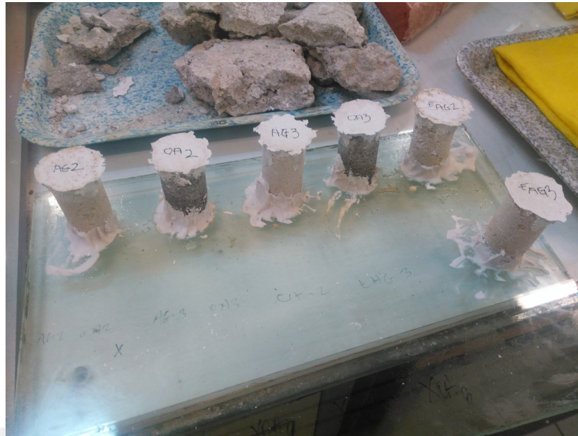
Fig. 3.28 : Plaster footings for preparing the samples for compression tests.
