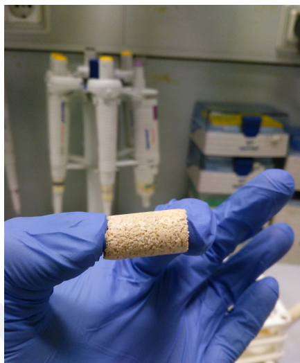
Fig. 3.10 : Successful cementation of a 5ml 1000-500µm sized Agora Beige sample.
