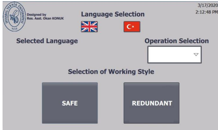
Figure 4.18 : The root screen of the designed HMI.
