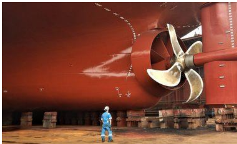
Figure 4.6 : Vessel after treatment of hull and polishing of the propeller [29].
