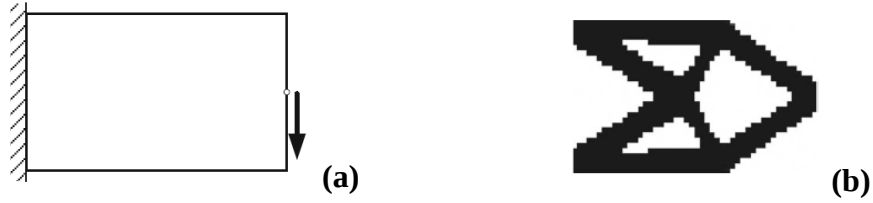
Figure 5.7 : Topology optimization process of a beam consisting of 48x30 elements (a) initial domain and (b) optimized design.
