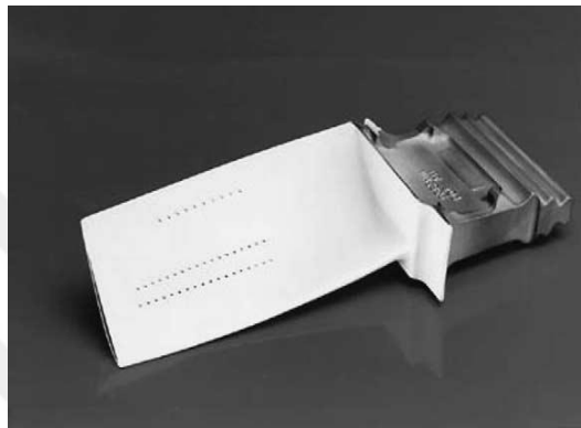
Figure 3.17 : General Electric CF6 turbine blade.
