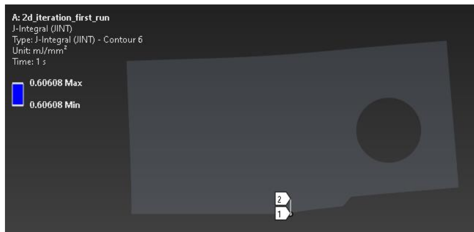
Figure 4.11 : Elastic J-Integral results of 2D elastic model.
