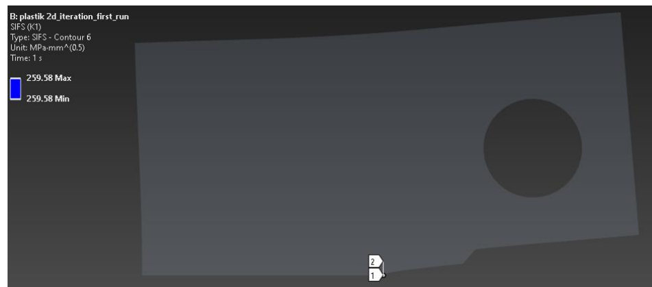
Figure 4.6 : The maximum stress intensity factor of 2d plastic model.
