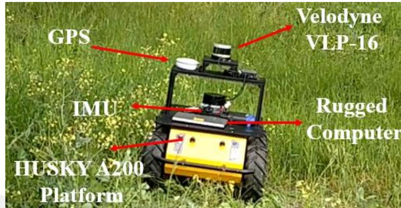
**Figure 5.2** : UGV experimental setup-outside.
