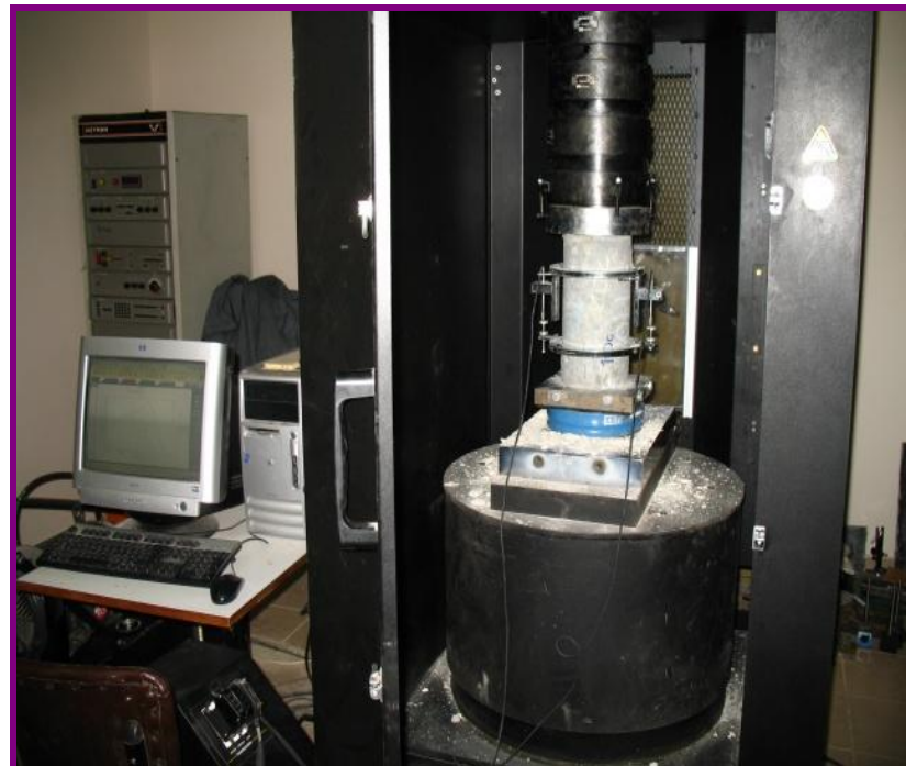
Figure 3.1: Testing machine (INSTRON 1000RD) with computerized data acquisition system
