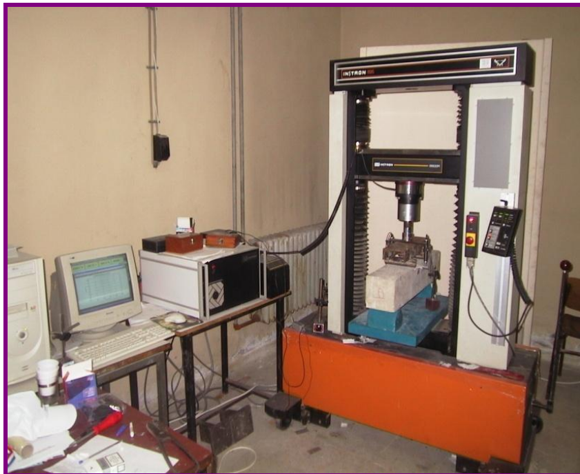
Figure 3.2: Bending testing machine (INSTRON 1195) with computerized data acquisition system
