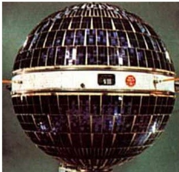
Figure 1.7 : Courier 1B with its many solar cells.
