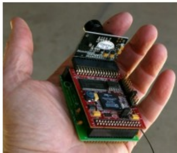
Figure 3.3 : SVR-1 kit, with AD Balckfin DSP and OV9655 CMOS sensor module.
