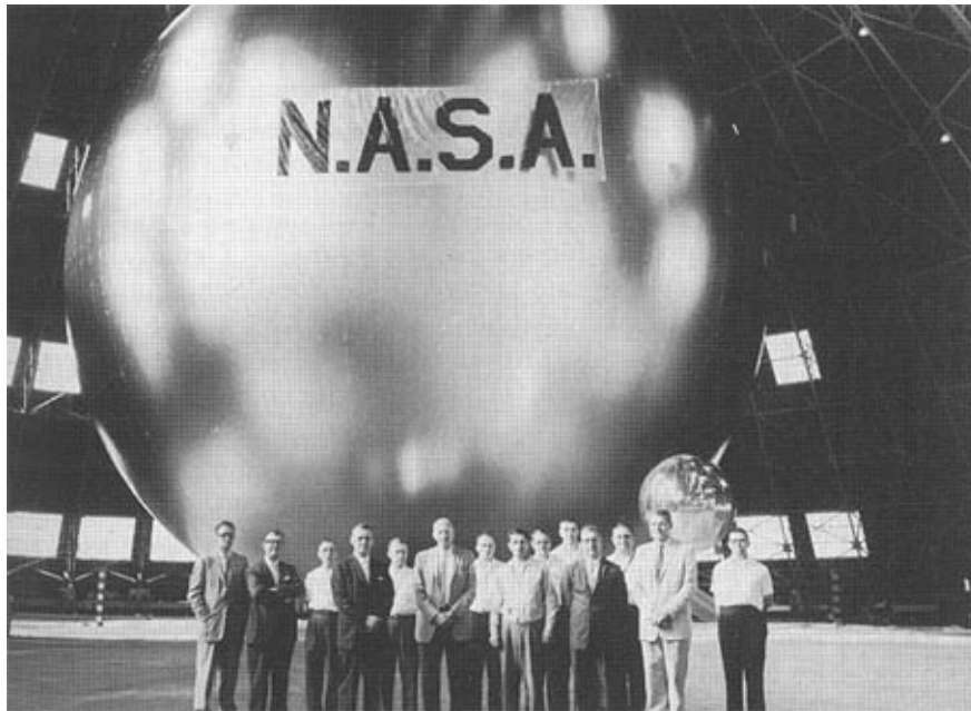
Figure 1.6 : Echo-1 was a balloon shaped satellite.
