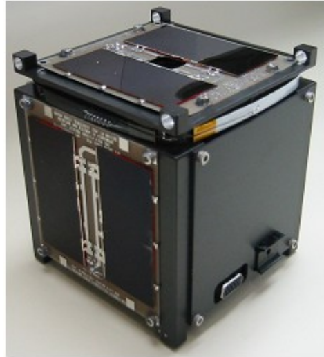
Figure 4.34 : CP-1 flight model.
