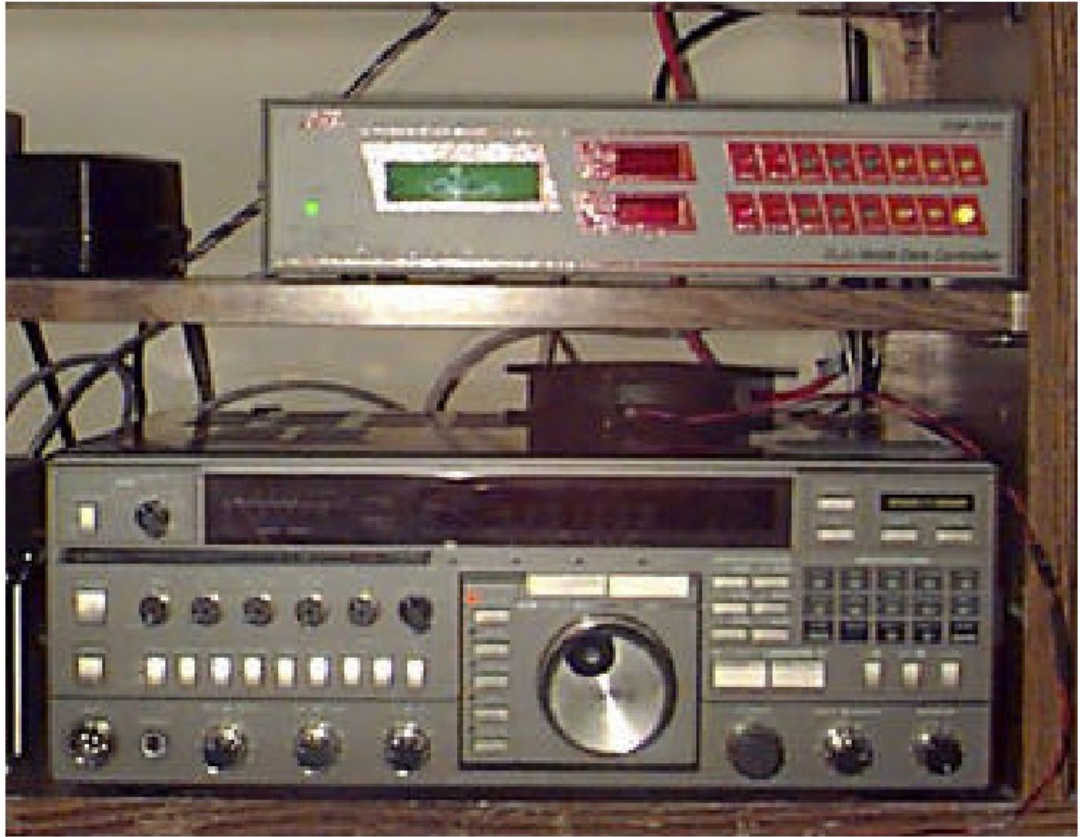
Figure 4.13 : Initial transceiver and TNC for ground station Mercury.
