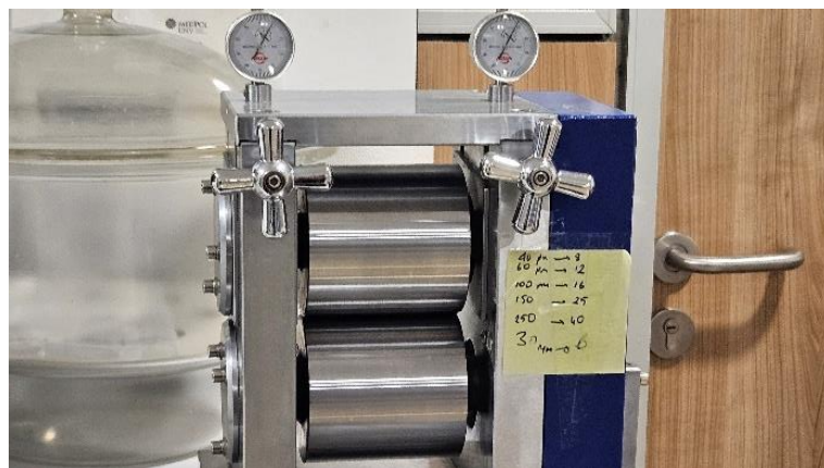
Figure 3.13 : Roll for rolling the electrode on copper foil to 30 \mu\text{m} thickness.
