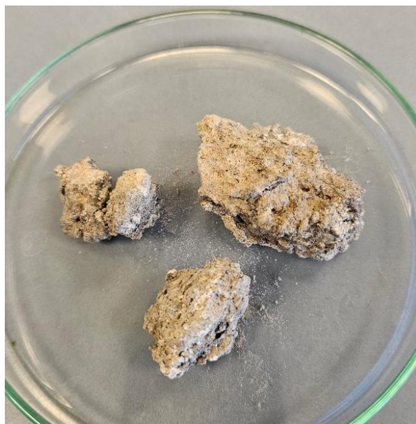
Figure 3.2 : Hot dip galvanizing dross.
