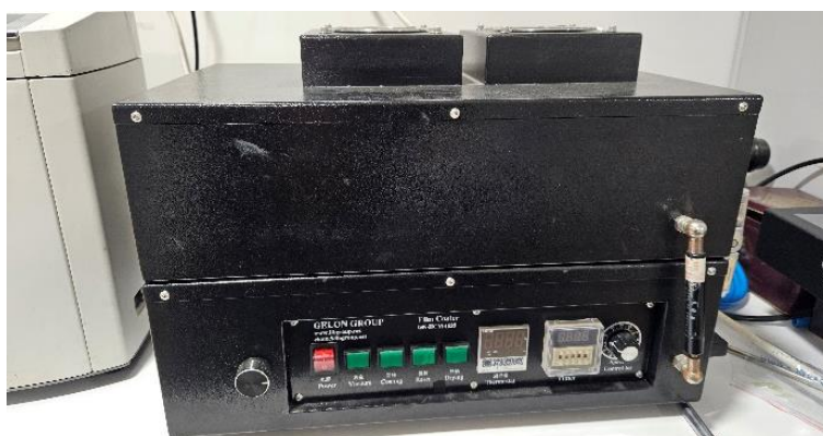
Figure 3.12 : Gelon Group Film Coater GN-HCM-1525 Doctor Blade.
