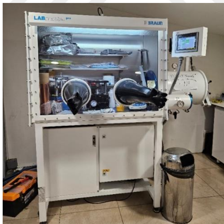
Figure 3.14 : MBRAUN LABMaster glove box.
