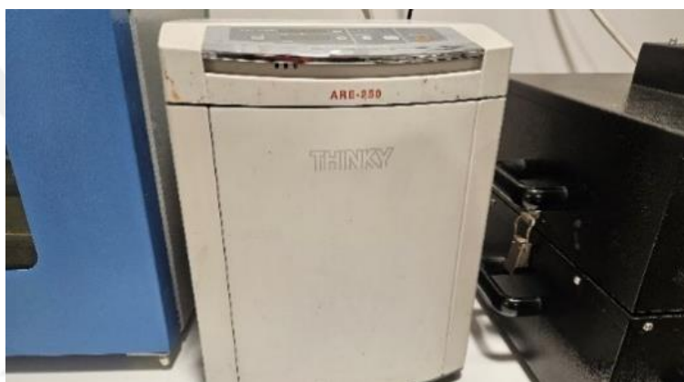
Figure 3.11 : Thinky ARE-250 for mixing the anode mixture.
