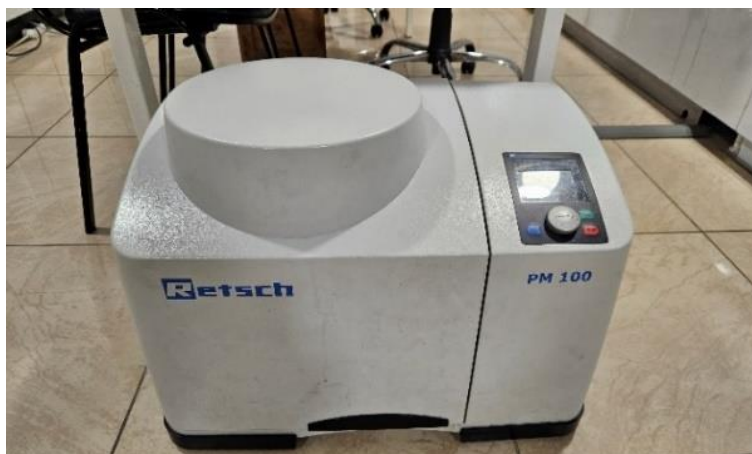
Figure 3.6 : Retsch PM 100 Planetary Ball Mill.
