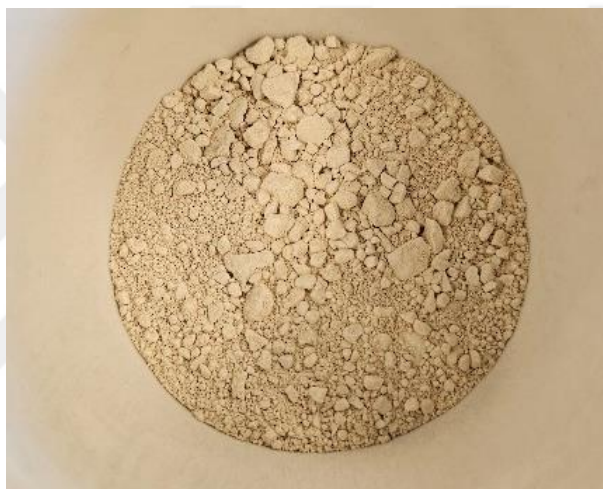
Figure 4.6 : Fe doped ZnO after heat treatment.
