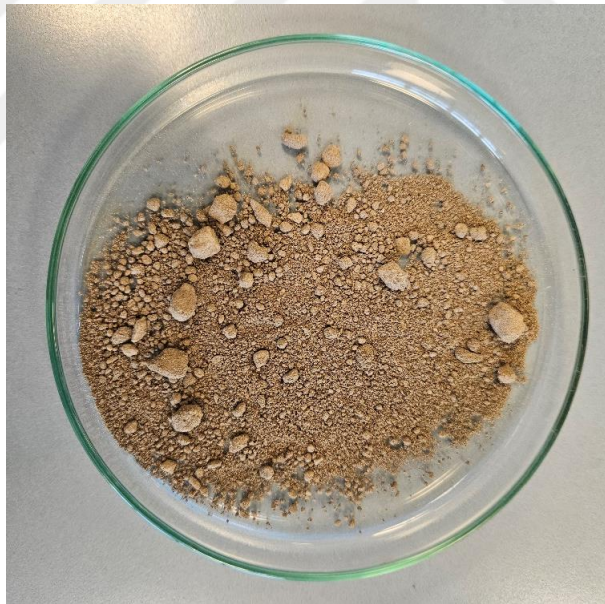
Figure 3.1 : Hot dip galvanizing flue dust.
