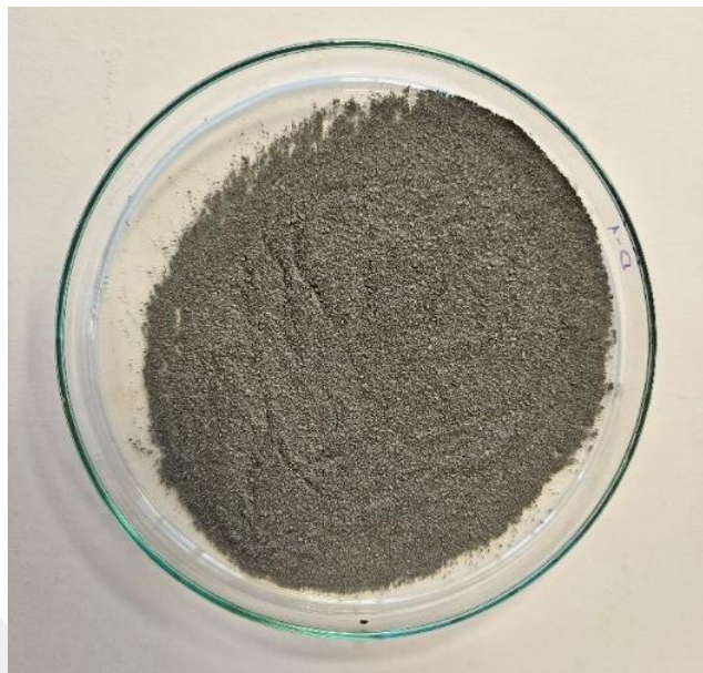
Figure 4.17 : Hot dip galvanizing dross after sieving with a 100 \mu\text{m} .
