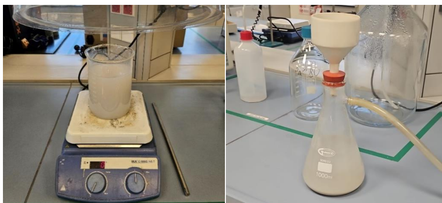
Figure 3.10 : Chemical precipitation with 0.5M (\text{NH}_4)_2\text{CO}_3 and filtration.
