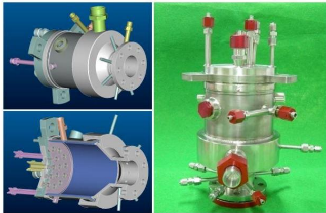
Figure 5.10: 30-tonf LPRE Gas Generator [7]
