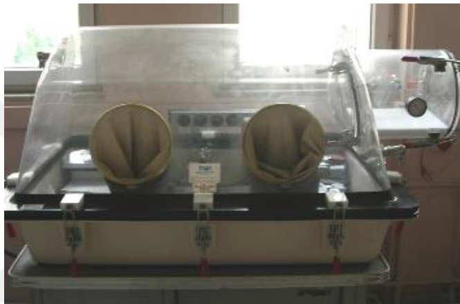
Figure 3.5 : Plas-Labs ™ glove box used while loading and unloading of the powders in to the vials (ITU Particulate Materials Laboratories, PML).
