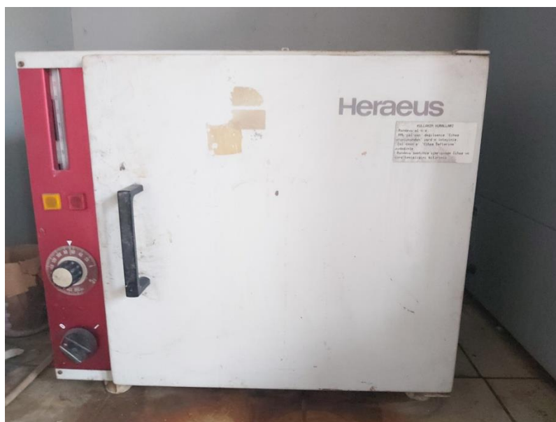
Figure 3.10 : Heraeus™ FN 500 stove (ITU Particulate Materials Laboratories, PML).
