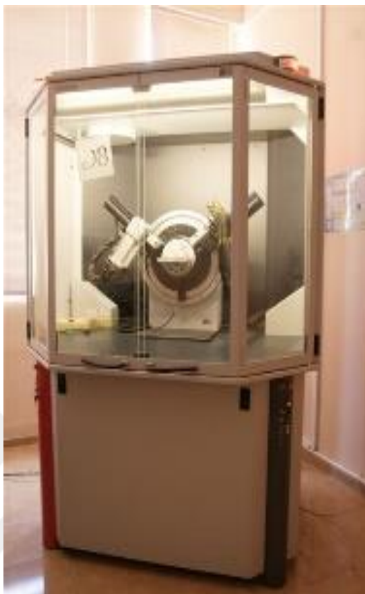
Figure 3.16 : Bruker™ D8 Advanced Series X-ray diffractometer (XRD) (ITU Particulate Materials Laboratories, PML).
