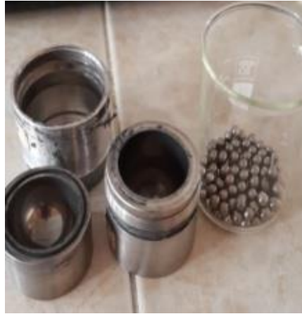
Figure 3.4 : WC vials and WC balls used in milling experiments.
