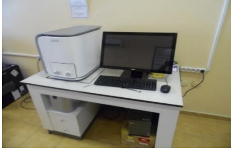
Figure 3.19 : JEOL™ JCM-6000 Benchtop Scanning Electron Microscope (SEM) (ITU Particulate Materials Laboratories, PML).
