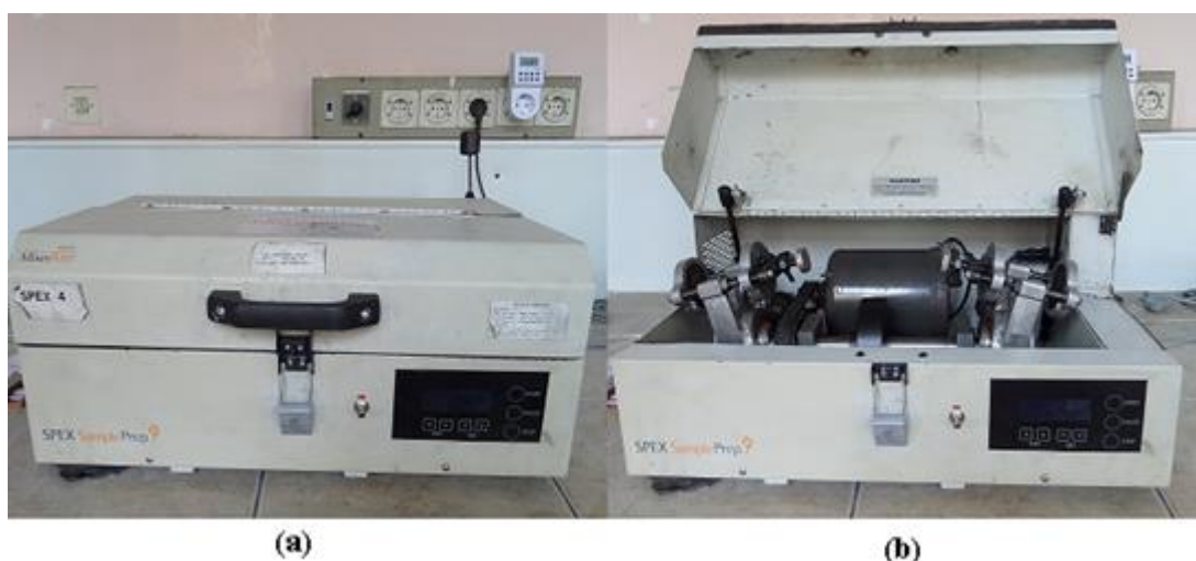
Figure 3.3 : Spex™ 8000 D Mixer/Mill in Particulate Materials Laboratories (PML) (a) lid closed and (b) lid opened.
