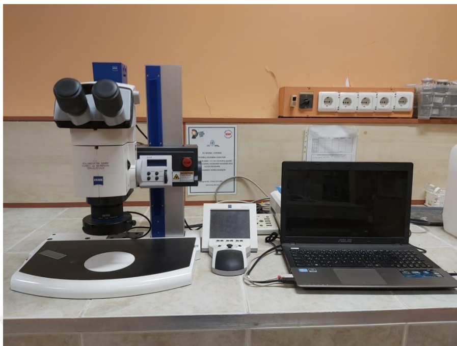
Figure 3.17 : Zeiss™ Discovery.V12 Stereomicroscope (SM) (ITU Particulate Materials Laboratories, PML).
