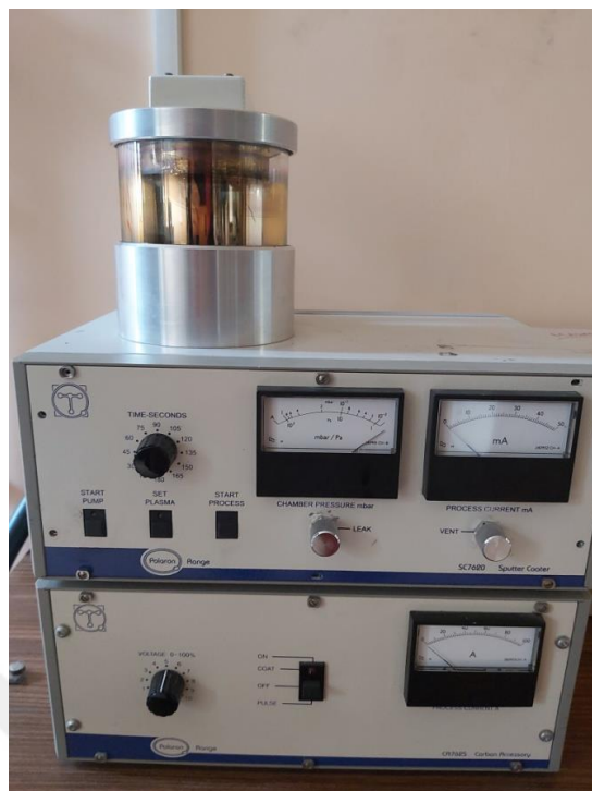
Figure 3.21 : Polaron™ SC7620 Sputter Coater (ITU Particulate Materials Laboratories, PML).
