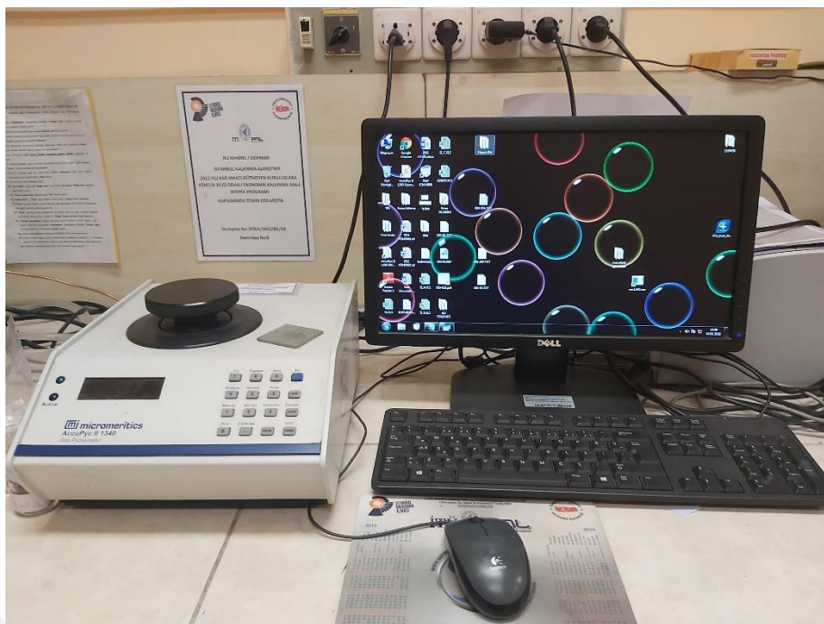
Figure 3.23 : Micromeritics™ AccuPyc II 1340 gas pycnometer (ITU Particulate Materials Laboratories, PML).
