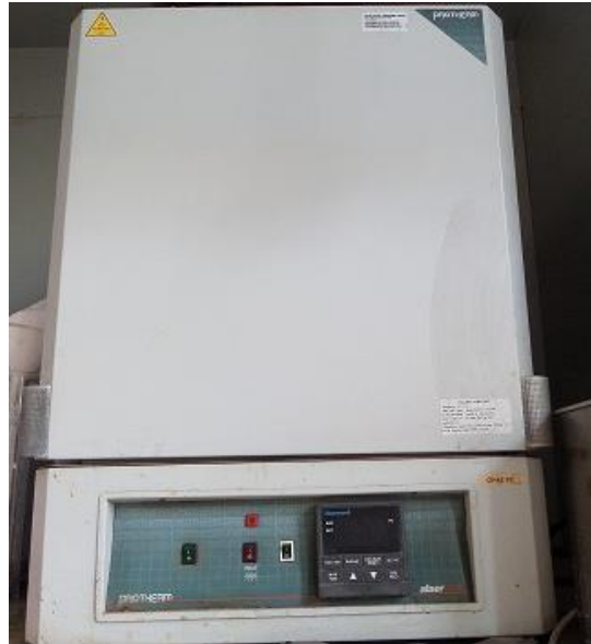
Figure 3.14 : Prothermal™ binder removal furnace into which hydrothermal reactor was placed (ITU Particulate Materials Laboratories, PML).
