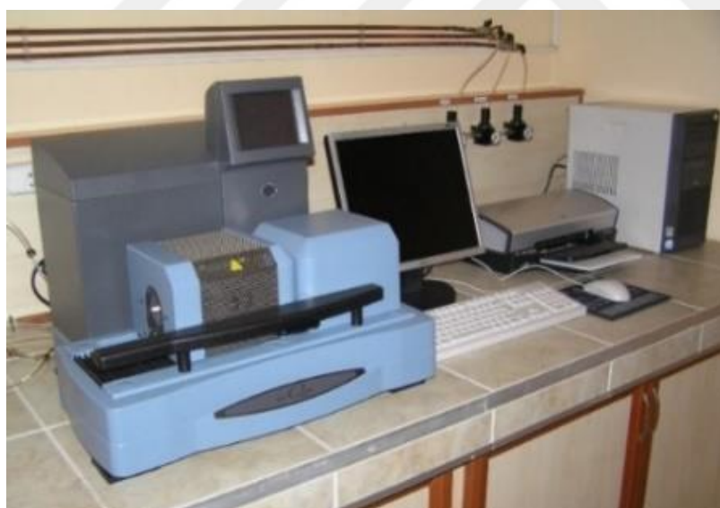
Figure 3.18 : Instruments SDT Q600 Differential Scanning Calorimeter (DSC)/Thermogravimetric Analyser (TGA) (ITU Particulate Materials Laboratories, PML).
