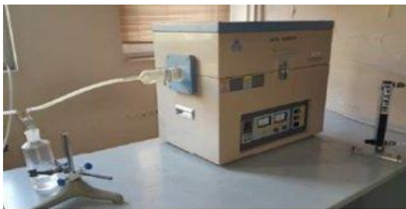
Figure 3.6 : MTI ™ QTF-1200X tube furnace used in sintering process (ITU Particulate Materials Laboratories, PML).
