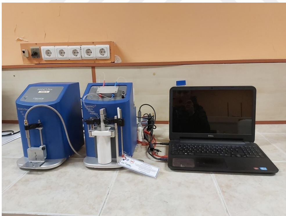
Figure 3.22 : Microtrac™ Nano-flex particle size analyzer (PSA) (ITU Particulate Materials Laboratories, PML).
