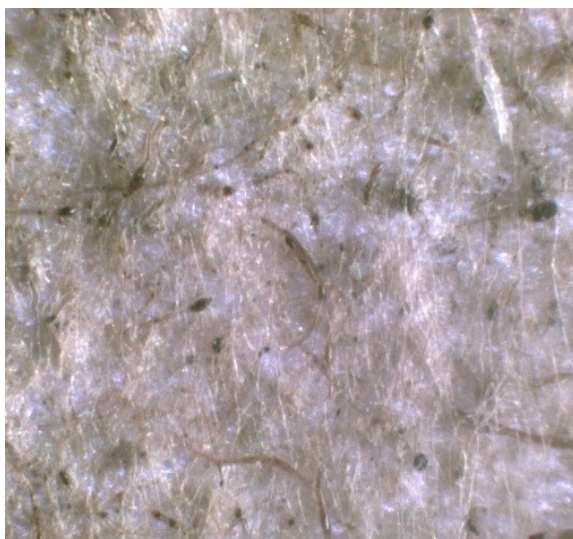
Figure 4.56 : Microscopic observation of nanofibers after modification with dye.
