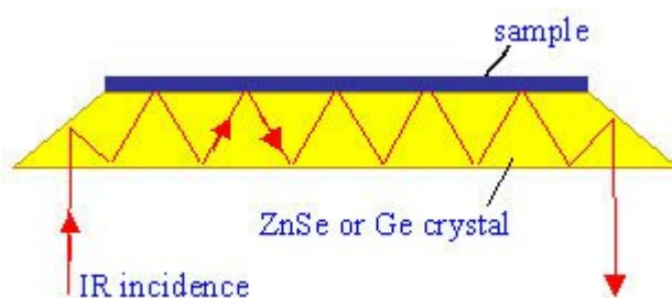
Figure 2.15: Working principle of FTIR-ATR [60].
