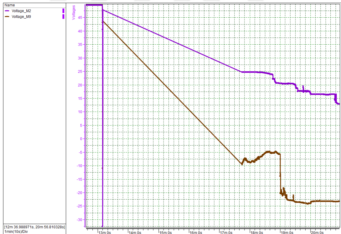
Figure 4.12: Trigger module and neighboring module voltages of attempt 1
