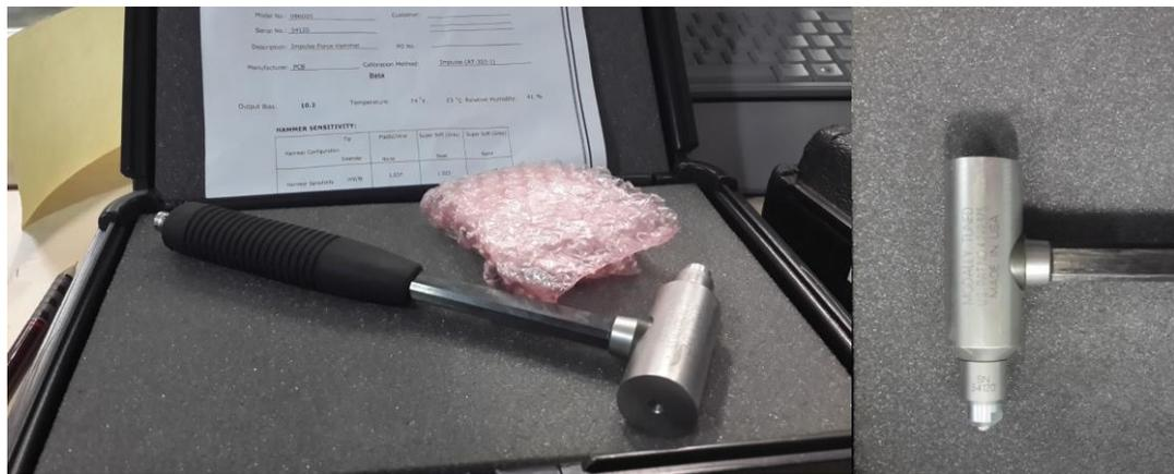
**Figure 5.4 :** Impact hammer used for the second test (hammer #2).
