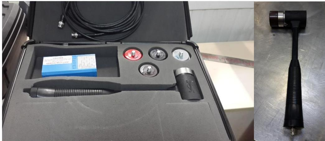
**Figure 5.3 :** Impact hammer used for first test (hammer #1) which was performed on HXXX steering wheel as attached to cab.
