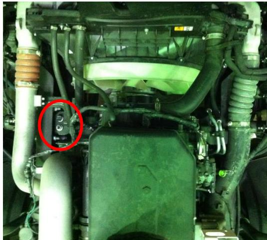
**Figure 4.1 :** Accelerometer placement on engine active side bracket.
