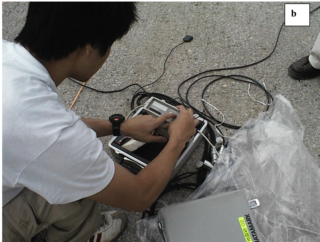
Figure 4.3. Some photos from the field work. (a) Arrangement of the stations of smallest array (2 m). (b) Arrangement of the signal conditioner and digitizer unit for the smallest array measurement.
