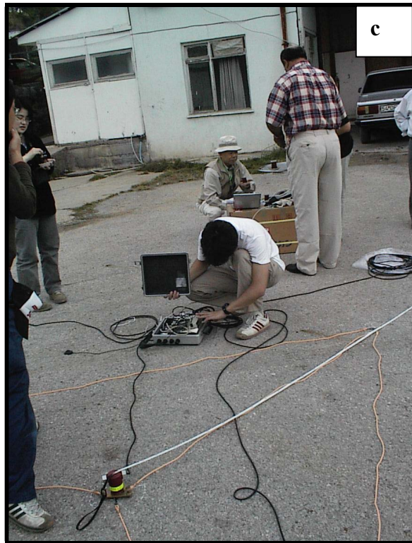
Figure 4.5. Some photos from the field instruments. (a) Triaxial accelerometer (b) Signal conditioner and data logger (c) General view of accelerometer, signal conditioner, data logger, computer and their connection.
