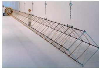
Fig. 12: Deployed FAST mast as used on ISS (Courtesy of Able Engineering – Extracted from [7])
