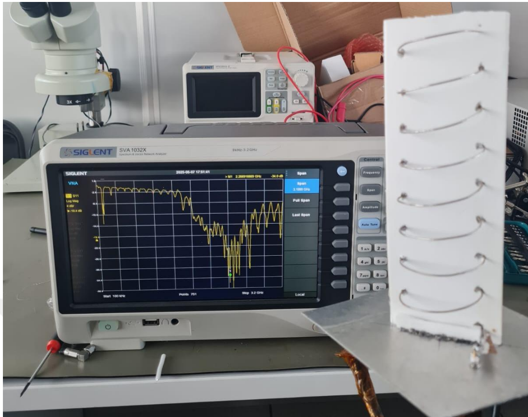
Figure 5.3 : Initial S11 spectrum testing of the antenna.
