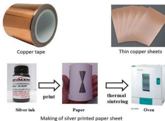
Figure 3.9 : Conductive materials for fabricating origami antennas.
