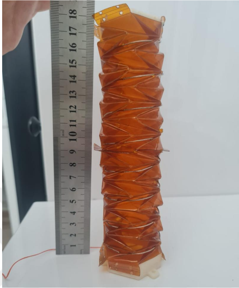
Figure 4.3 : Deployed version of antenna (176 mm).
