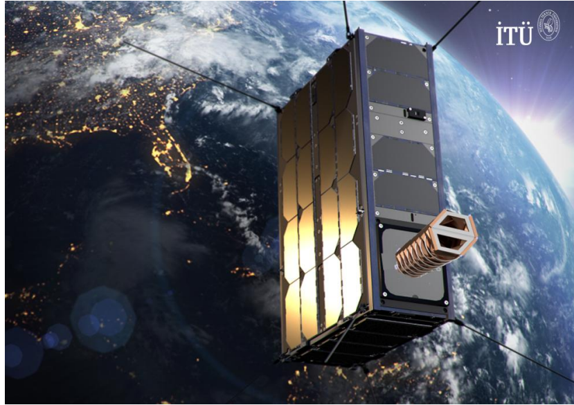
Figure 4.13 : Rendering of deplored version of helical origami antenna with 6U CubeSat configuration.
