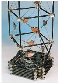
Fig. 11: Beginning deployment of ADAMmast (Source: NASA)
