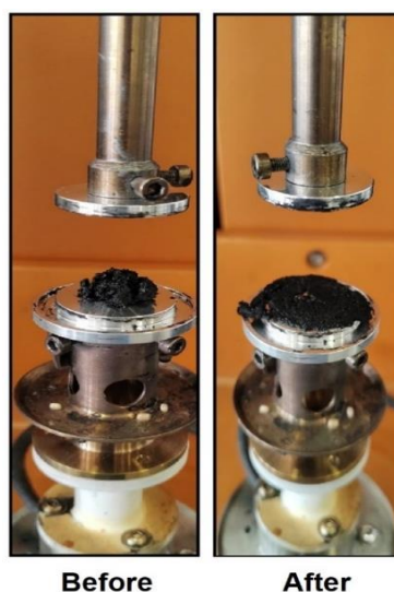
Figure 4.9 : CNTNC/CNC 6.0:6.0 (water/IPA 70/30) before and after steady state test.
