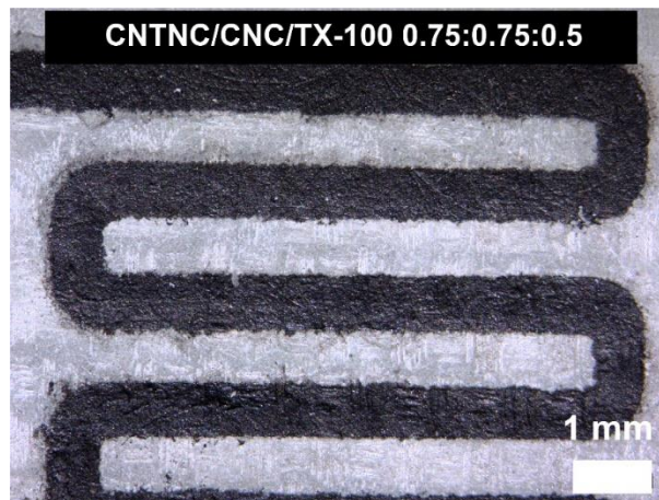
Figure 4.36 : Light microscope image of the spray-printed sensor using an 8-layer CNTNC/CNC/TX-100 0.75:0.75:0.5 ink formulation, exhibiting well-defined edges, uniform deposition, and minimal defects.
