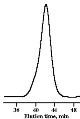
Figure 4.2. GPC trace of epoxy chain end functionalized macromonomer ( 4 )
