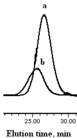
Figure 4.8. GPC trace of PSt ( 8 ) (a) and PSt-g-PCHO graft copolymer ( 18 ) (b) (Table 4.5, Run 3).
