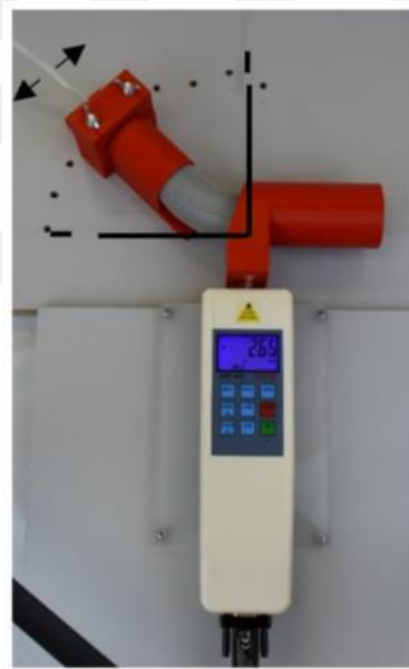
Figure 6.4: Output torque measurement setup.
