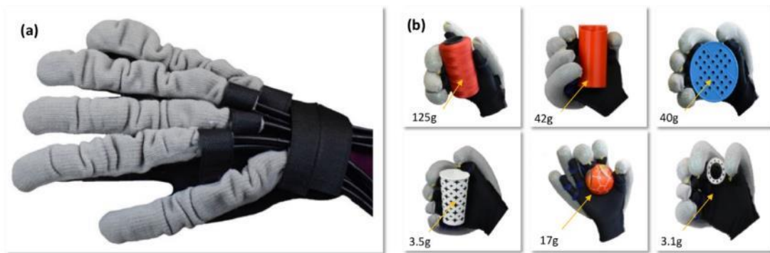
Figure 6.6: (a) Wearable assistive glove prototype based on a seamless knitted actuator. (b) Achievable motions with the glove prototype for grasping objects of different weights and sizes.
