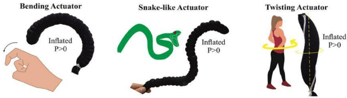
Figure 5.1: The novel method provided to create bio-inspired bending, snake-like, and twisting actuators.
