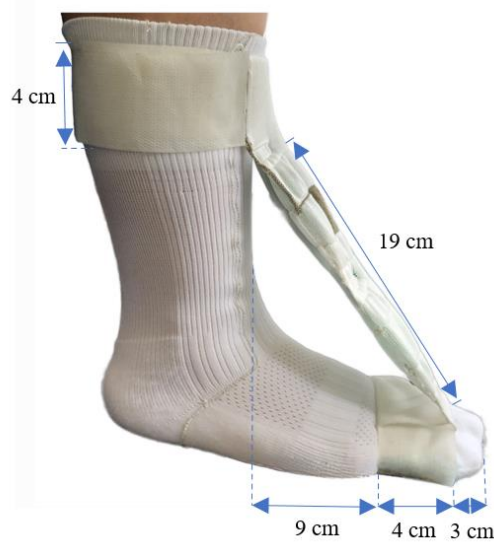
Figure 3.6: Attachment points of the knitted pouch motor to the foot and ankle.
