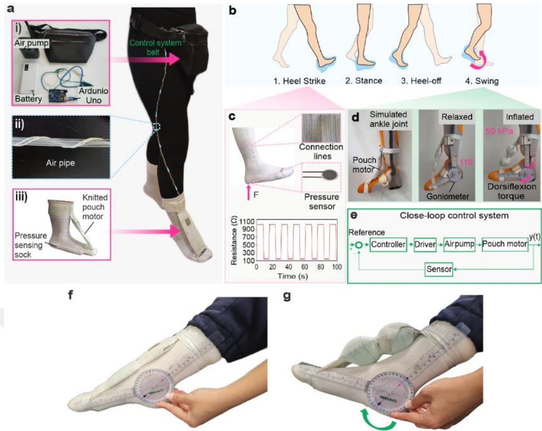
Figure 3.10: Application demonstration of the soft pouch motor in assistive robotics. (a) Showing the concept behind the soft ankle-foot orthosis exosuit. (b) Phases of the human gait. (c) Functionality and application of the textile-based resistive pressure sensing sock. (d) Dorsiflexion motion of the simulated ankle joint by soft pouch motor. (e) Close-loop control block diagram. (f) Deflated pouch motor fastened to a human foot. (g) Dorsiflexion of the human foot using pouch motors that is inflated.
